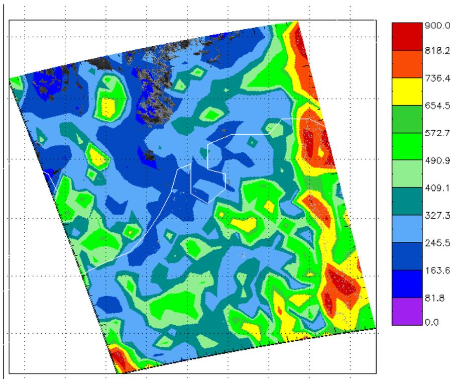
Figure 5.16: Cloud Liquid Water Path for water clouds in g/m-2, 3 December 2001
