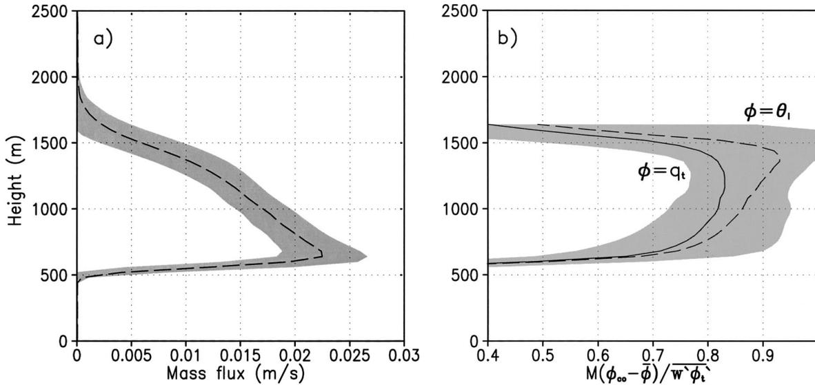
FIG. 8. (a) The mass flux profile of the core ensemble, and (b) the ratio between the turbulent flux  $\overline{w'\phi'}$  and its mass flux approximation  $M(\phi_{co} - \bar{\phi})$  [see (9)], based on the LES results for  $\phi = q_t$  (solid) and  $\phi = \theta_t$  (dashed).
