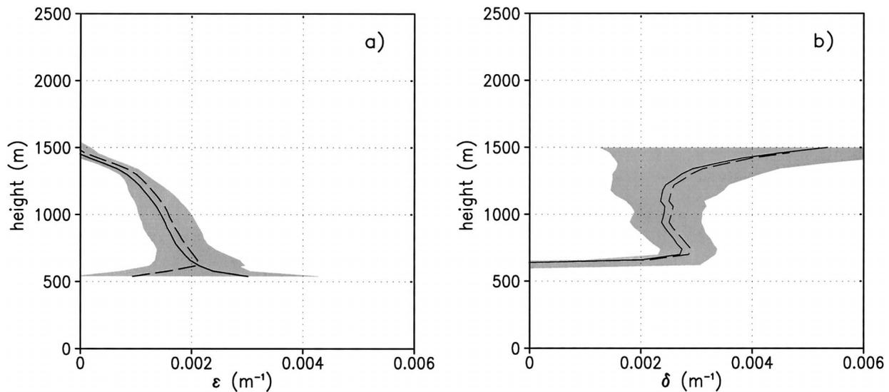
FIG. 9. Fractional entrainment rate  $\epsilon$  and detrainment rate  $\delta$  diagnosed using (10)–(11) for  $\phi = q_t$  (solid line) and  $\phi = \theta_t$  (dashed line).
