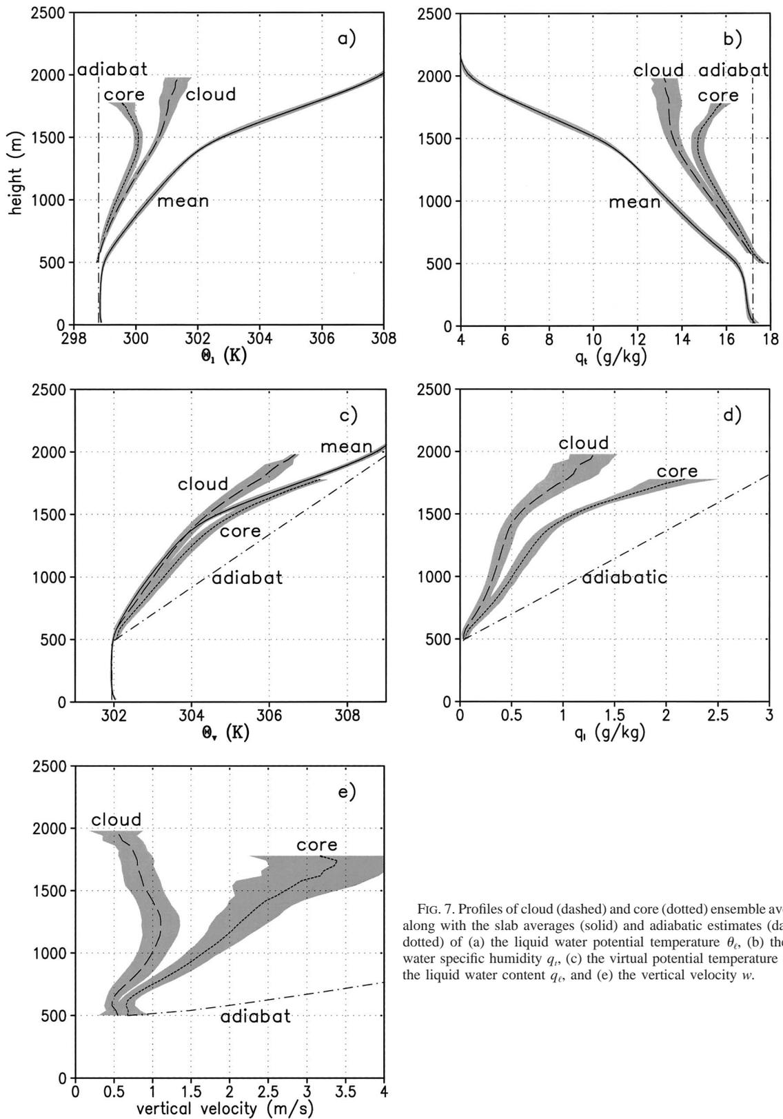
FIG. 7. Profiles of cloud (dashed) and core (dotted) ensemble averages along with the slab averages (solid) and adiabatic estimates (dashed-dotted) of (a) the liquid water potential temperature  $\theta_l$ , (b) the total water specific humidity  $q_t$ , (c) the virtual potential temperature  $\theta_v$ , (d) the liquid water content  $q_l$ , and (e) the vertical velocity  $w$ .
