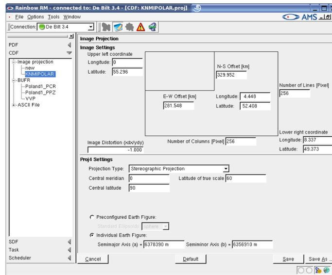
Figure 3.9: Snapshot from the Rainbow 5 radar product processor of the window where the geographical projection can be defined.
