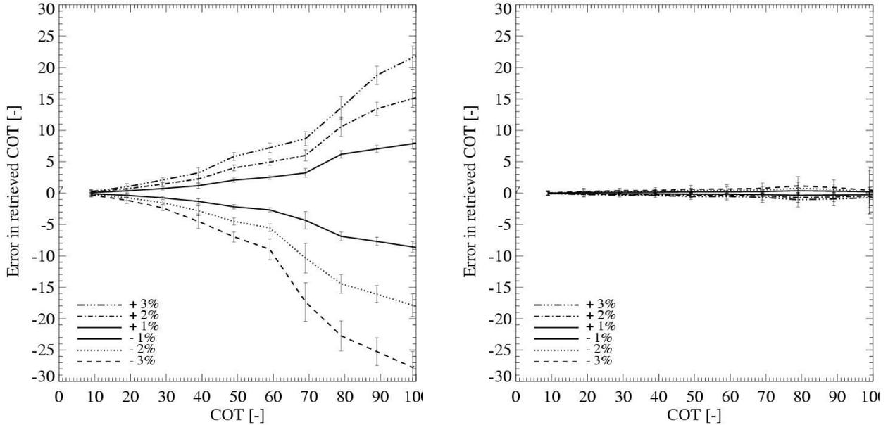
FIG. 10. Error in retrieved cloud optical thickness (-) assuming errors of  $\pm 1$ , 2 and 3% in the 0.63 (left) and 1.61  $\mu\text{m}$  (right) reflectances. The error bars represent differences due to the iteration and interpolation scheme.
