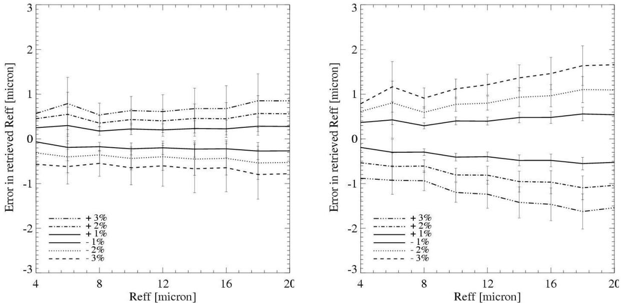
FIG. 11. Error in retrieved droplet effective radius ( $\mu\text{m}$ ) for water clouds with  $\tau > 4$  assuming errors of  $\pm 1$ , 2 and 3% in the 0.63 (left) and 1.61  $\mu\text{m}$  (right) reflectances. The error bars represent differences due to the iteration and interpolation scheme.
