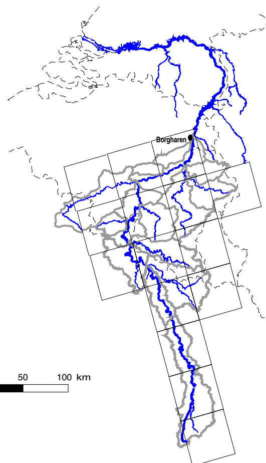
Figure 1 Locations of the 15 RACMO grid boxes used in this study, relative to the Meuse subbasins (thick grey contours) and the river Meuse with tributaries. State boundaries (dashed) and the location of the gauging station Borgharen are also shown.
