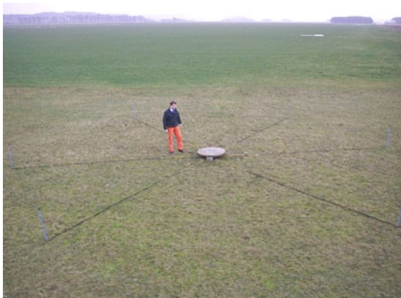
Figure 4.2: The field installation of a micro-barometer with noise reducer attached constructed of soaker hose. The micro-barometer is mounted beneath the earth's surface for temperature stability and robustness.
