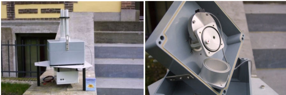
Figure 4.1: The KNMI micro-barometer; a differential pressure sensor based on Validyne pressure transducer.
