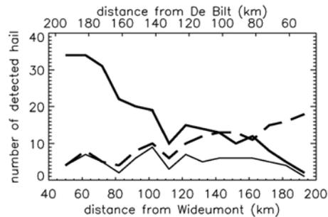
Fig. 3: Number of detected hail cases as a function of range for the radars of Wideumont (solid line) and De Bilt (dashed line). The thin solid line shows the number of hail cases detected by both radars.
