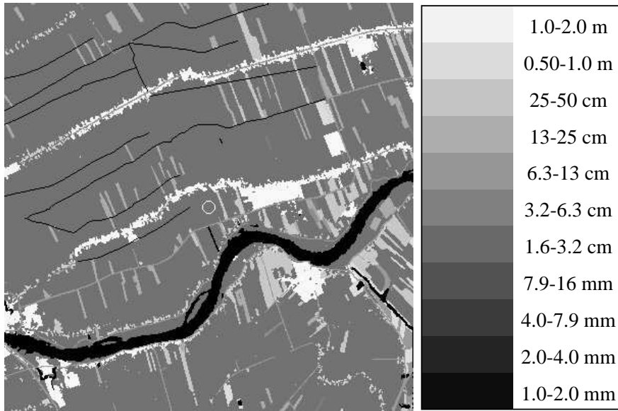
Figure 1. Roughness lengths in gray scale for the Cabauw environment [(10 \text{ km})^2] . The circle in the center of the figure indicates the tower position. Dark areas are smooth, bright areas are rough. Lowest and highest roughness lengths found in this region are approximately 0.001 and 1 m respectively. Pixel size (25 \text{ m})^2 .
