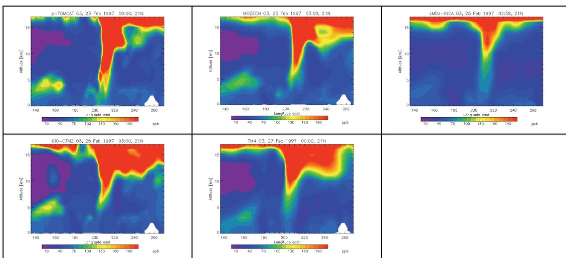
**Figure 3:** Vertical cross sections of ozone along 21°N on the 25<sup>th</sup> of February 1997, 03:00 h GMT. Top row from left to right: p-TOMCAT, MOZECH, LMDz-INCA, bottom row: UiO-CTM2 and TM. Note that p-TOMCAT results are for 00:00 h GMT and TM results are a 24-hour average.
