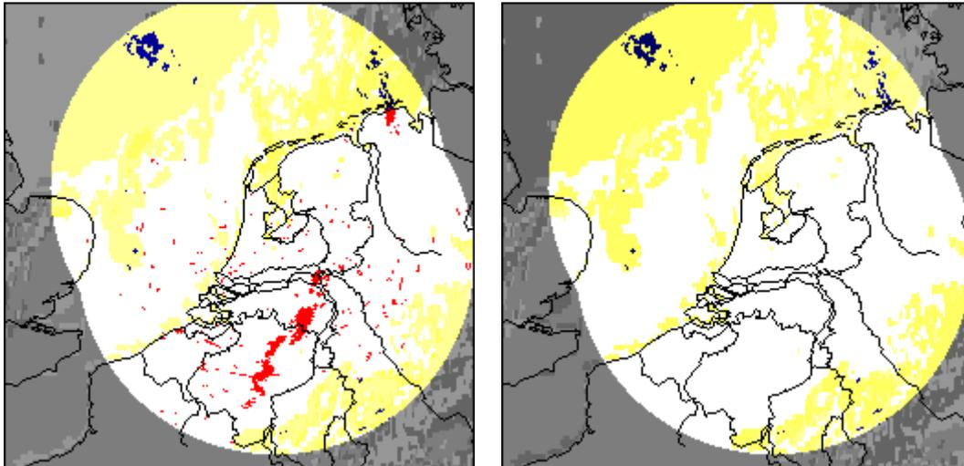
**Figure 2.** June 8, 2006, 12:00 hr GMT. Composite of the KNMI radar ETH product in red (clutter) and blue merged with the SAFNWC cloud mask, represented in white as cloud free and yellow as cloudy. The coloured area within the grey area indicates the radar coverage. Left is the original image and right is the filtered radar product.
