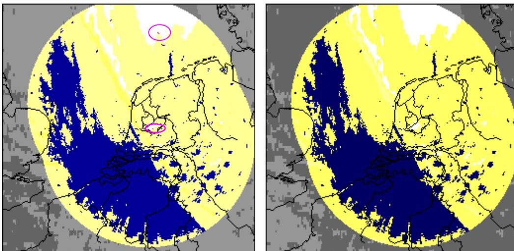
**Figure 3.** Caption as in Figure 2 but for June 1, 2006, 12:00 hr. Only two clutter cases could be identified indicated by the purple ellipses. Please note the attenuation at the South West of the radar product.
