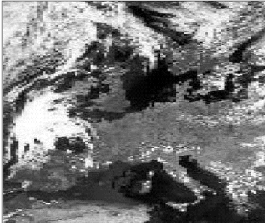
Fig. 4.5 AVHRR channel 2 image over Europe resampled to a grid of approximately 13 \times 40 \text{ km}^2 , to give an impression of the required spatial resolution for OMI.
