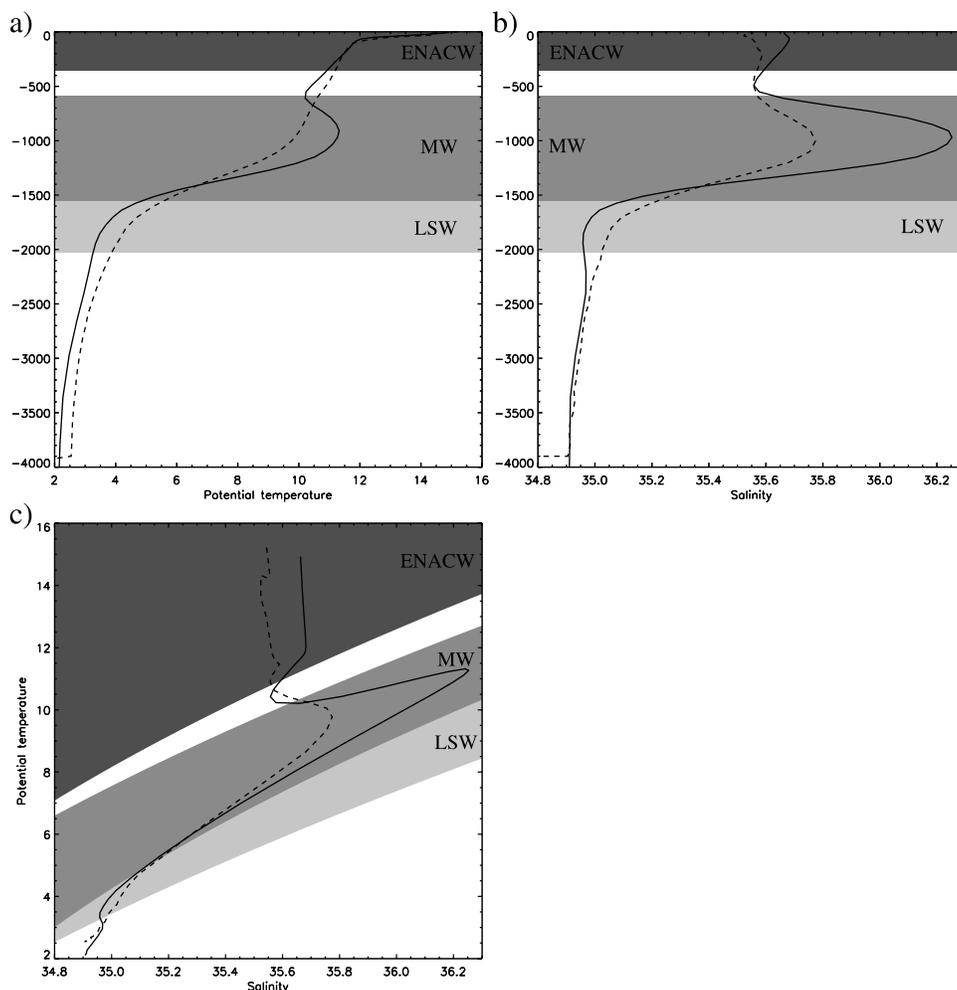
**Figure 2.** Mean climatological ( $\Theta$ ,  $S$ ) properties in the model (solid line) compared to the *Reynaud et al.* [1998] climatological data set (dashed line): (a) Mean temperature and (b) mean salinity profiles over the Biscay abyssal plain; (c) ( $\Theta$ ,  $S$ ) diagram over the Biscay abyssal plain; the density ranges of Eastern North Atlantic Central Water (ENACW), Mediterranean Water (MW), and Labrador Sea Water (LSW) are shaded.
