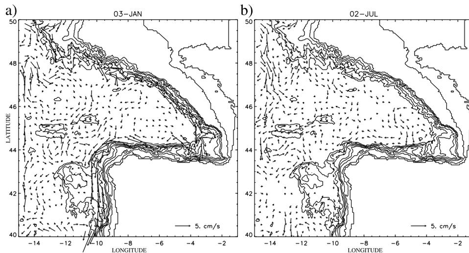
**Figure 11.** Snapshots of climatological velocity vectors averaged in depth between 1400 m and 1600 m at 6-month time intervals: (a) Early January; and (b) early July. Velocities smaller than  $0.2 \text{ cm s}^{-1}$  are not shown.
