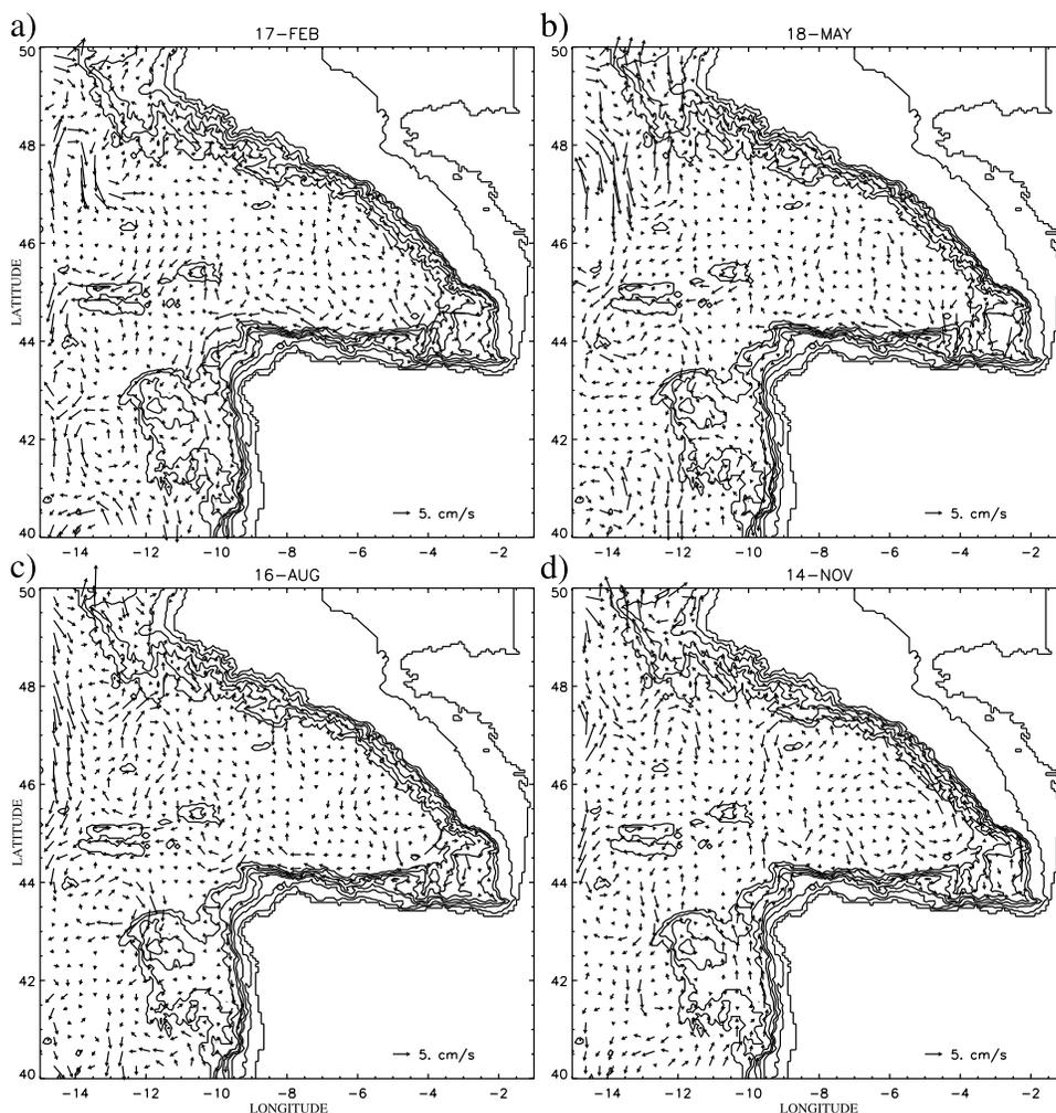
**Figure 7.** Snapshots of climatological velocity vectors averaged in depth between 350 m and 520 m at 3-month time intervals: (a) Mid-February; (b) mid-May; (c) mid-August; and (d) mid-November. Velocities smaller than  $0.2 \text{ cm s}^{-1}$  are not shown.
