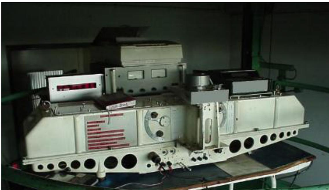
Figure 2: The Dobson instrument nr 40 at Uccle, Belgium.
