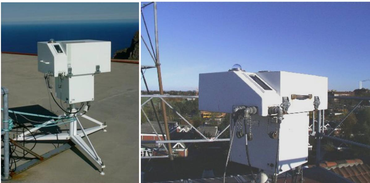
*Figure 4: SCI-TEC Brewer ozone spectrophotometer (MK-III type) on the roof of ALOMAR, Norway (left) and Brewer ozone spectrophotometer (MK-II type) in Copenhagen, Denmark (right).*
