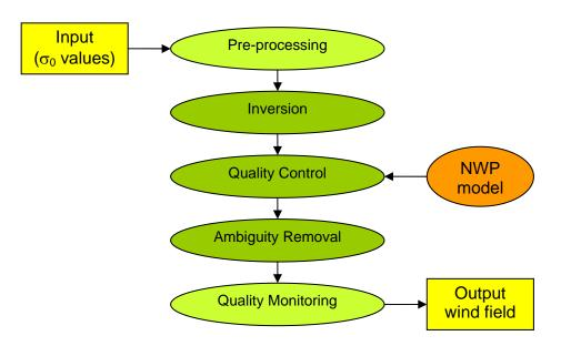
Figure 2: Schematic view of KNMI scatterometer wind processing software
