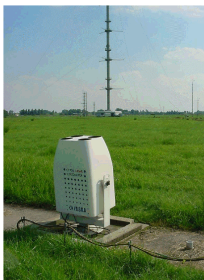
FIGURE B.3.8 Vaisala CT75K lidar ceilometer at the Cabauw site.
