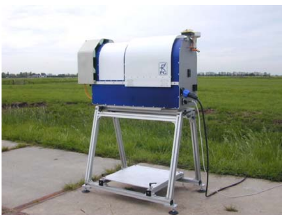
FIGURE B.3.9 Low-cost HATPRO radiometer, used in the Integrated Profiling Technique.
