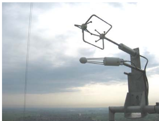
FIGURE B.3.6 Sonic anemometer installed by Alterra at the 100 m level of the mast.
