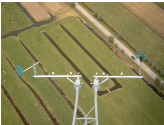
FIGURE B.3.5 Wind vane and cup anemometer in the Cabauw mast.
