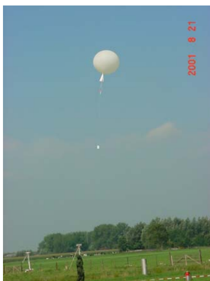
FIGURE B.3.7 Launch of a RS90 sonde during the BBC1 campaign.
