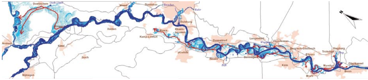
..... Figure 10.1 Flooding along the Lower Rhine between Bonn (right) and Arnhem (left). Red arrows indicate the direction of the spreading of the flood. The flooded area is shown in light blue. After Lammersen and Kroekenstoel (2005).
