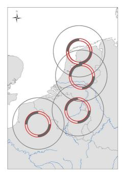
Figure 7: Area of the Flysafe nucleus. The large circles denote the maximum detection range for birds (150 km) of the four military long-range surveillance radars. Standardized measurement windows (50-60 km range, 90-180 and 270-360 degrees azimuth) for quantitative bird densities are indicated by dark grey segments.
