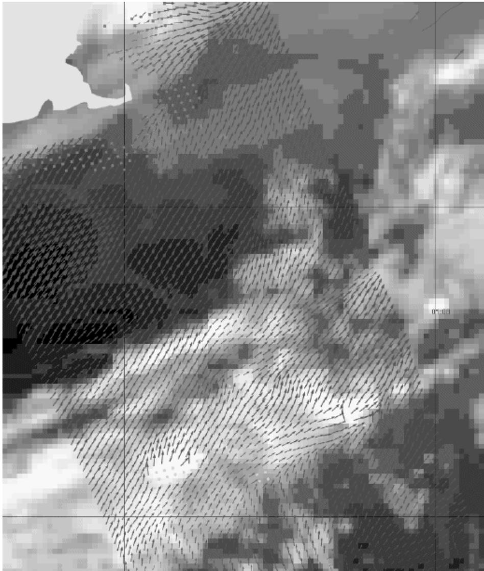
**Figure 2:** Experimental ASCAT 12.5-km wind product generated at KNMI on top of collocated GOES IR cloud imagery underneath. Centered at 38N, 68W, on 4 July 2008 00:30 Z.
