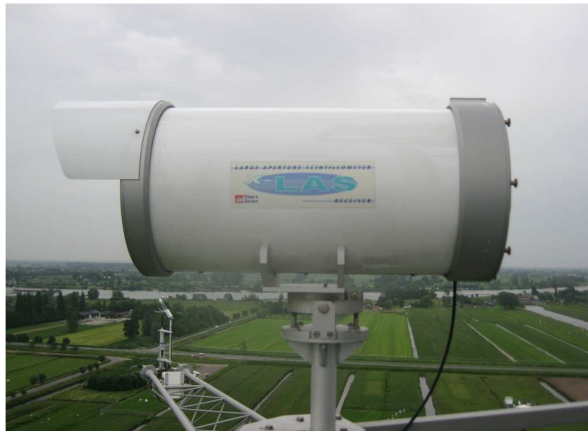
Figure 3 The receiver of the scintillometer at the Cabauw Tower at 61.7 m.
