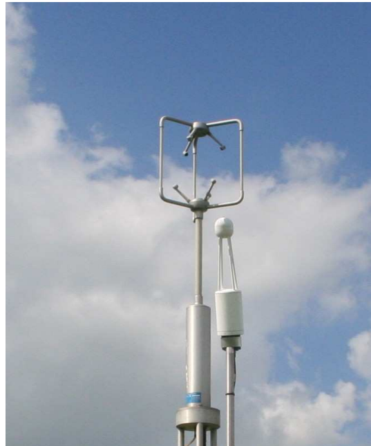
Figure 2 The sonic anemometer/ thermometer at 3 m.
