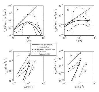
**Figure 2.** SGF defined by (25) as a function of the droplet radius for the wind speed (a) 20 m s<sup>-1</sup> and (b) 30 m s<sup>-1</sup>. (c) Total droplets surface area and (d) droplets volume fluxes as a function of the friction velocity. Lines: see legend. Thin solid lines with a number n on the top indicate the wind dependence  $u_n^n$ .
