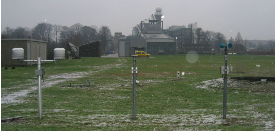
Figure 4: Instruments at the operational site DB260. To the left the KNMI multi-plate radiation shield for measuring temperature and to the right the cup anemometer. Both instruments operate at 1.5 m above ground level. The 4 parallel locations are equipped with the same instruments.
