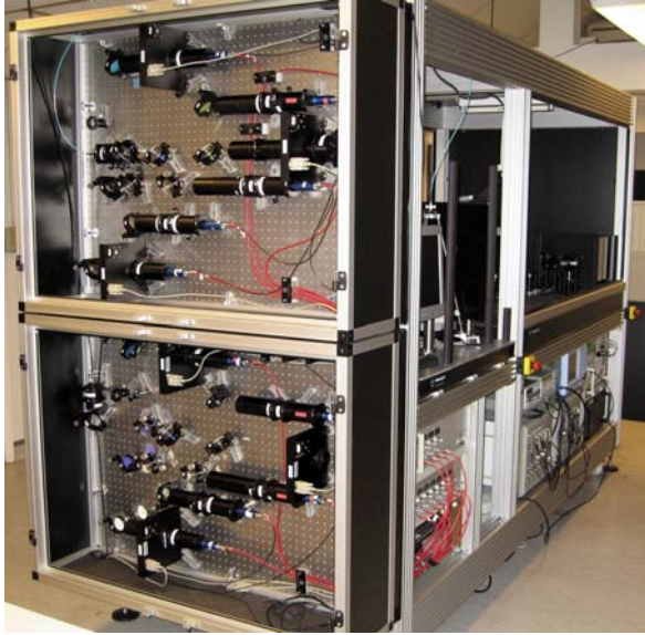
Figure 2. Caeli framework ( 3 \times 1.2 \times 2 \text{ m}^3 ) before mounting to the container. The NFR (top) and FFR (bottom) receiver sections are normally closed, but now exposed for the picture. Electronics and computers are situated below the emitter optical table.
