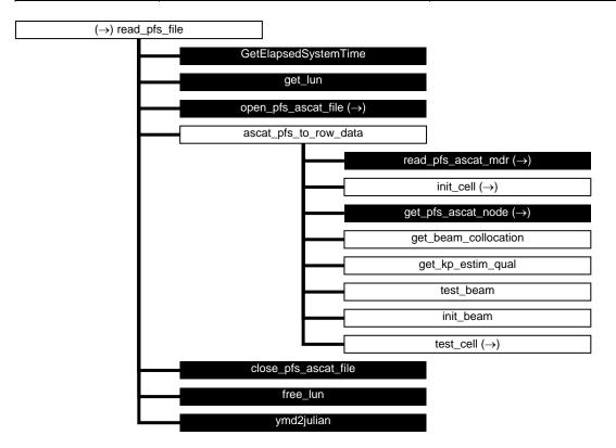
**Figure A.3** Calling tree for routine *read\_pfs\_file* (first level).
