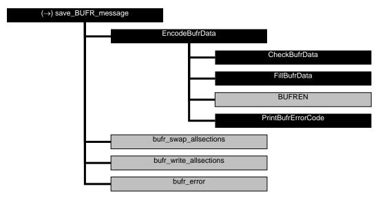
**Figure B3.4** Calling tree for BUFR file handling routine *save\_BUFR\_file*.
