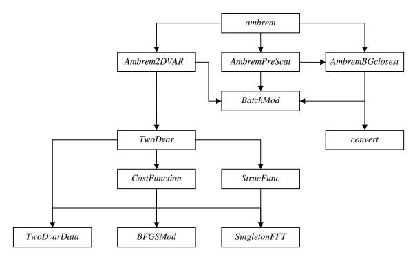
**Figure 6.1** Interdependence of the modules for Ambiguity Removal. The connections from module *ambrem* to module *BatchMod* and from module *Ambrem2DVAR* to *convert* are not drawn.
