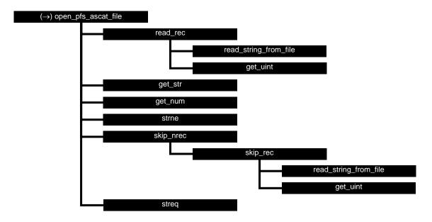
**Figure B5.1** Calling tree for PFS file handling routine *open\_pfs\_ascat\_file*.
