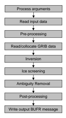
Figure 4.1 Baseline of the ASCAT Wind Data Processor
