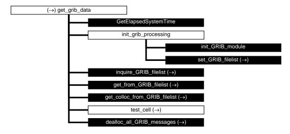
**Figure A.6** Calling tree for routine *get\_grib\_data* (first level).
