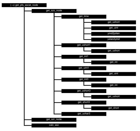
**Figure B5.3** Calling tree for PFS file handling routine  $get\_pfs\_ascat\_node$ . The calling tree for  $get\_szr\_node$  is identical to to the one of  $get\_szo\_node$ .
