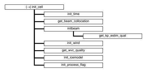
**Figure A.12** Calling tree for routine *init\_cell* (second level).
