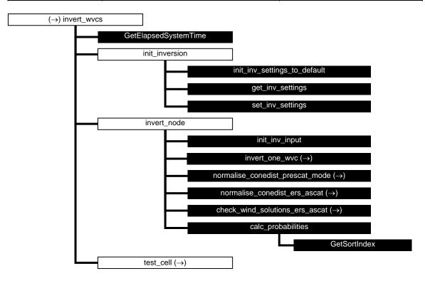
**Figure A.7** Calling tree for routine *invert\_wvcs* (first level).
