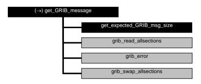
**Figure B4.6** Calling tree for GRIB file handling routine *get\_GRIB\_message*.
