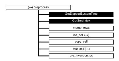
Figure A.4 Calling tree for routine *preprocess* (first level).
