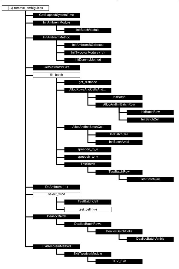
**Figure A.9** Calling tree for routine *remove\_ambiguities* (first level). The full name of the 12<sup>th</sup> routine is *AllocRowsAndCellsAndInitBatch*.
