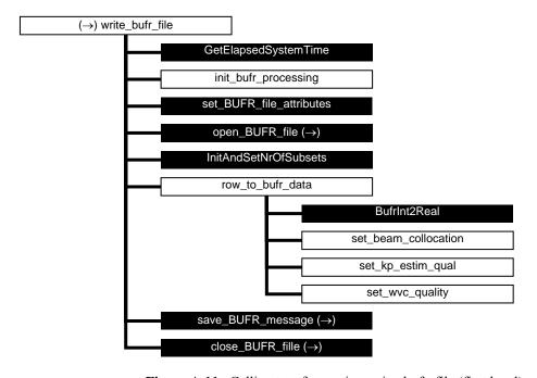
**Figure A.11** Calling tree for routine write\_bufr\_file (first level).
