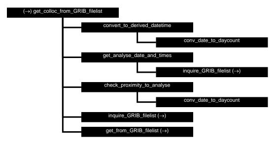
**Figure B4.4** Calling tree for GRIB file handling routine *get\_colloc\_from\_GRIB\_filelist*.
