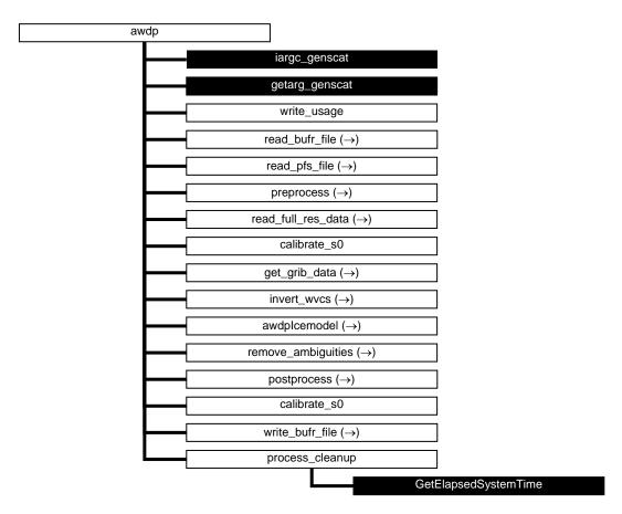
**Figure A.1** Calling tree for program *awdp* (top level). White boxes are cut here and will be continued in one of the first level or second level calling trees in the next figures. Black boxes with light text indicate genscat routines.
