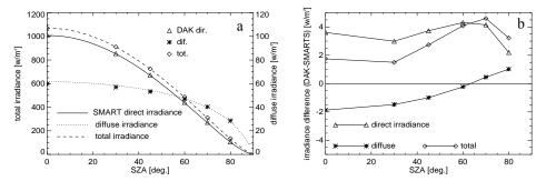
**FIGURE 2.** (a) DAK and SMARTS simulated direct, diffuse and total irradiances for s pure Rayleigh atmosphere. (b) The differences (DAK-SMARTS).
