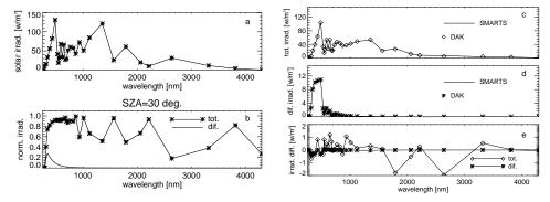
**FIGURE 1.** Left: (a) Solar spectrum at TOA at 32 wavelength bands. (b) DAK simulated total and diffuse irradiance spectra. The spectra are normalized. Right: DAK and SMARTS simulated (c) total irradiance spectra, (d) diffuse irradiance spectra, and (e) the differences. All the simulated spectra are at SZA= 30°.
