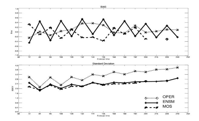
Fig. I Verification results for the operational (OPER), the ensemble mean (ENSM) and the Model Output Statistics (MOS) 2meter temperatures in terms of mean error (top) and standard deviation (bottom).
