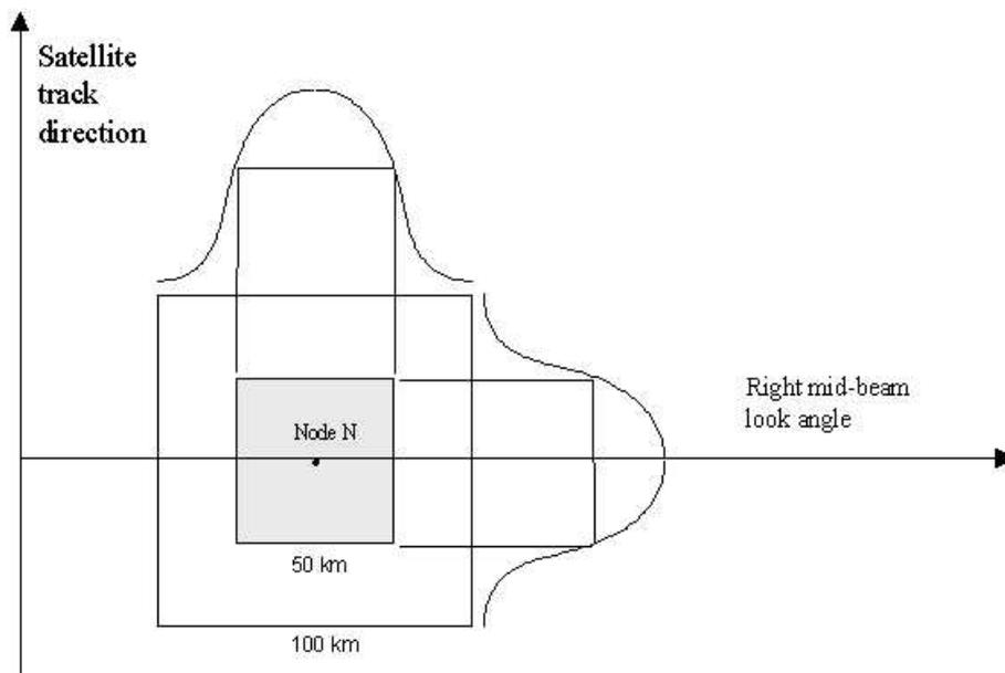
**Figure 3** Illustration of the Level 1 processing at each Node N for the 25-km ASCAT product (courtesy EUMETSAT).
