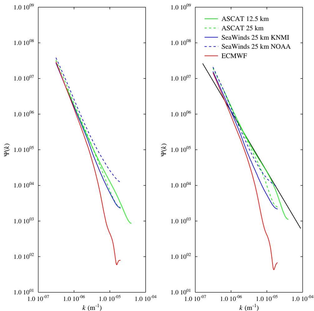
**Figure 2:** Spectra for the wind components  $u$  (left) and  $v$  (right) for ASCAT (green curves), SeaWinds (blue curves) and the ECMWF model (red curves). The black solid line in the right panel shows a  $k^{-5/3}$  spectrum.
