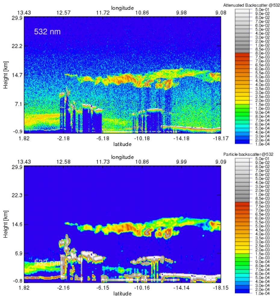
**Figure 2:** CALIOP L1 attenuated backscatter (top) and KNMI derived particle backscatter at 3.5km horizontal and 125 m vertical sampling (bottom), both at 532 nm. While noise artifacts are suppressed, the main atmospheric structures as observed by CALIOP are still visible in the lower panel. Regions of spurious artifacts below dense clouds will not be observed by Aeolus.
