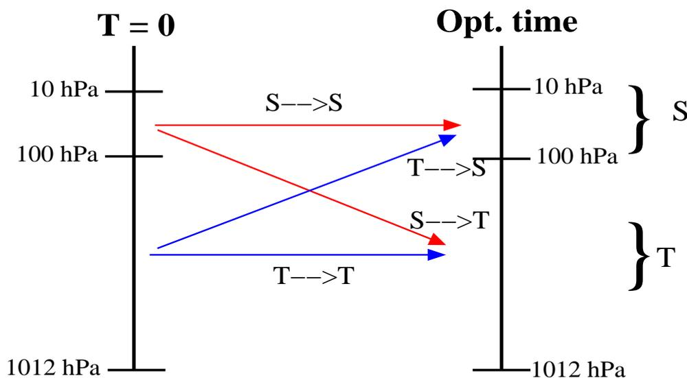
**Figure 4:** Illustration of the sensitivity experiments to test the linear evolution of initial stratospheric (S) or tropospheric (T) perturbations to either the stratosphere (S) or troposphere (T) at the optimization time.
