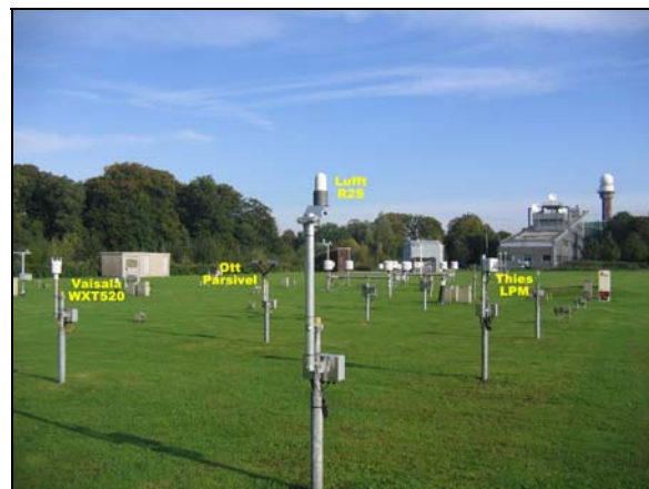
Figure 6: The test field in De Bilt, with the four precipitation type sensors under test indicated in the foreground.
