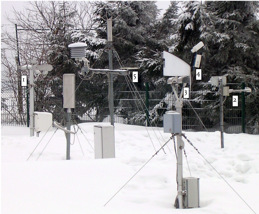
Figure 1. The PW sensors at Wasserkuppe, 25 February 2004. 1: Vaisala FD12P, 2: 2 Thies laser precipitation monitors (disdrometers), 3: Parsivel disdrometer (in front), 4: Metek micro rain radar. Also visible 5: Thies precipitation detector.
