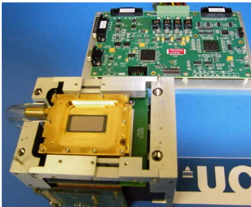
Figure 6-7: INO microbolometer sensor and control electronics for testing at UCL-MSSL
