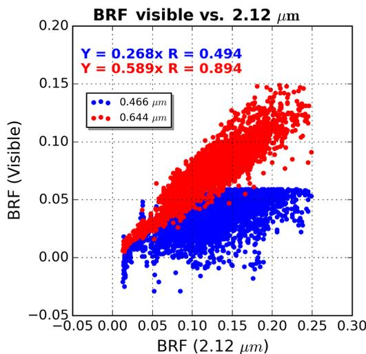
**Figure 3.** The BRF ratios of visible (0.466 and 0.644  $\mu\text{m}$ ) to 2.12  $\mu\text{m}$  wavelength, filtered by the dark surface under AOD < 0.2. The ratios are obtained by forcing linear regressions through the origin.
