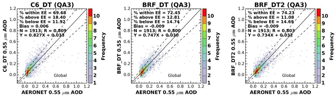
**Figure 12.** DT AOD validation over the global land. The DT algorithms are C6\_DT, BRF\_DT and BRF\_DT2. The retrieved AOD is filtered with QA = 3 (labeled as QA3), shown against AERONET AOD. The dash and solid line are expected error (EE)  $\pm(0.05 + 15\%)$  and one-one line, respectively.
