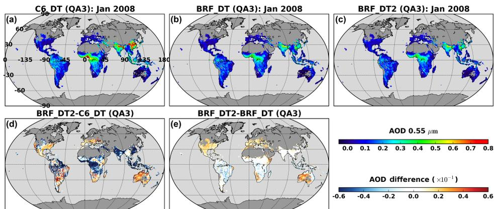
**Figure 7.** January 2008 maps (1° × 1°) of mean AOD filtered with the best-quality QA = 3 (labeled as QA3) over global land. (a–c) show the AOD retrieved from C6\_DT, BRF\_DT and BRF\_DT2, respectively. (d) and (e) show the AOD difference of BRF\_DT2–C6\_DT and BRF\_DT2–BRF\_DT, respectively.
