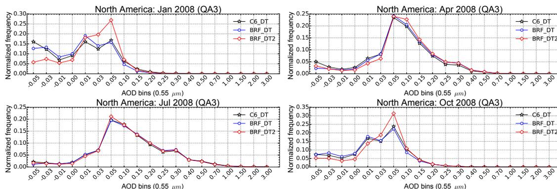
**Figure 9.** Histograms for North America DT AOD (at  $0.55 \mu\text{m}$ ) from Aqua for 4 months. Plotted are data from C6\_DT, BRF\_DT and BRF\_DT2 with QA = 3, labeled as QA3. Bin labels represent the lower boundary of the bin. For example, a bin labeled as  $-0.05$  means the AOD between  $-0.05$  and  $-0.03$ .
