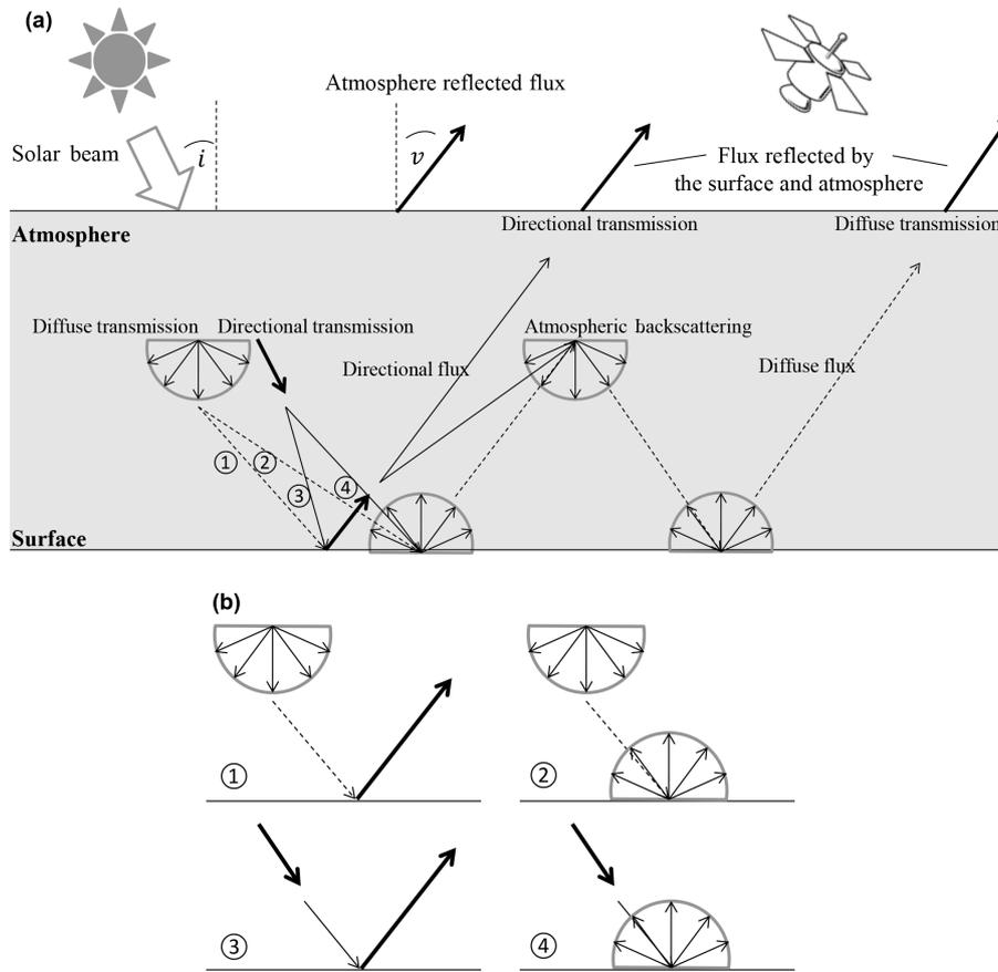
**Figure 2.** The TOA flux observed by the satellite considering the surface BRDF effects. The surface BRDF is simply described as four elements: hemispherical-directional (1), bihemispherical (2), bidirectional (3) and directional-hemispherical reflectance/reflection (4), also shown in panel (b). More details are explained in the text.
