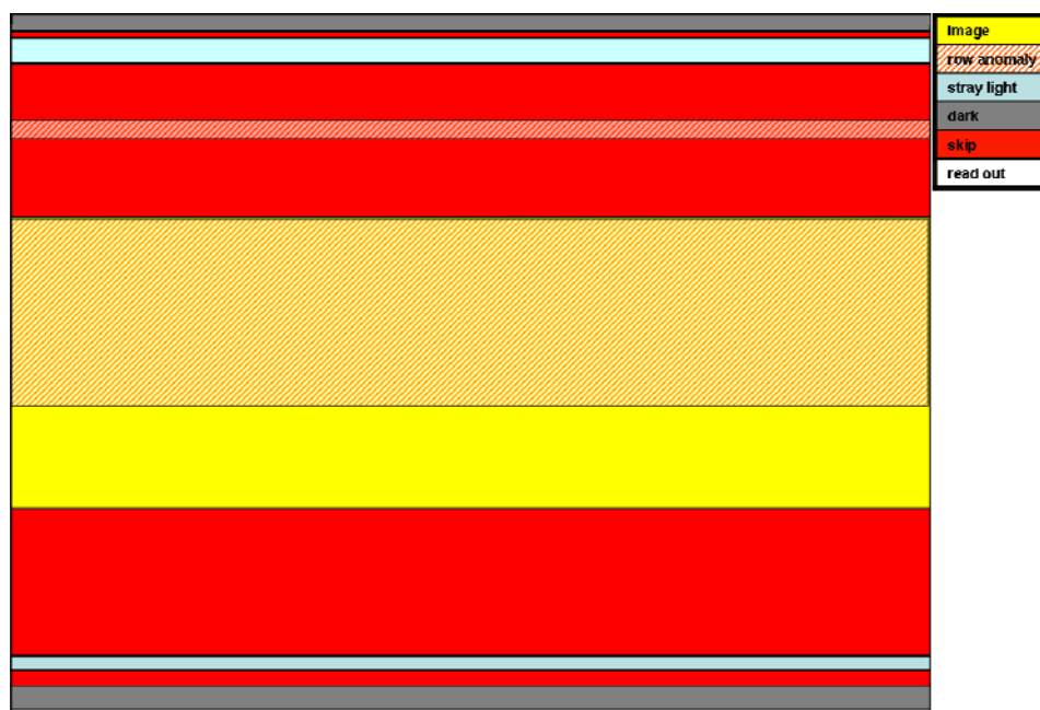
Figure 2. Current spatial zoom-in CCD settings. Indicated are the image area (yellow) (240 unbinned rows (60 binned rows (BF4))) and the area affected by the row anomaly (hatched). The row anomaly affects in this case 160 unbinned rows (40 binned rows (BF4)) in the image area. This is more than half (67%) of the image area.
