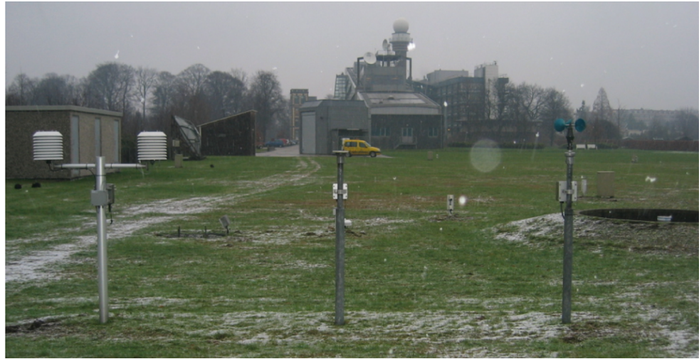
Figure 2.5: Instruments at DB260. The left side shows the KNMI multi-plate radiation shields for measuring temperature and relative humidity. The right side shows the cup anemometer. Both instruments operate at 1.5 m above ground level. The 4 parallel sites are equipped with the same instruments and have an identical set-up.
