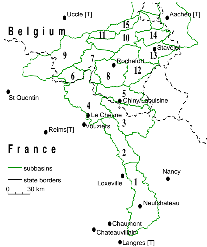
Figure 2.1: Location of stations in and around the Meuse basin and the definition of the HBV subbasins.
