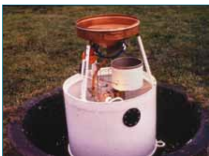
Figure 3.1. Example of a self-recording rain gauge (without lid).
