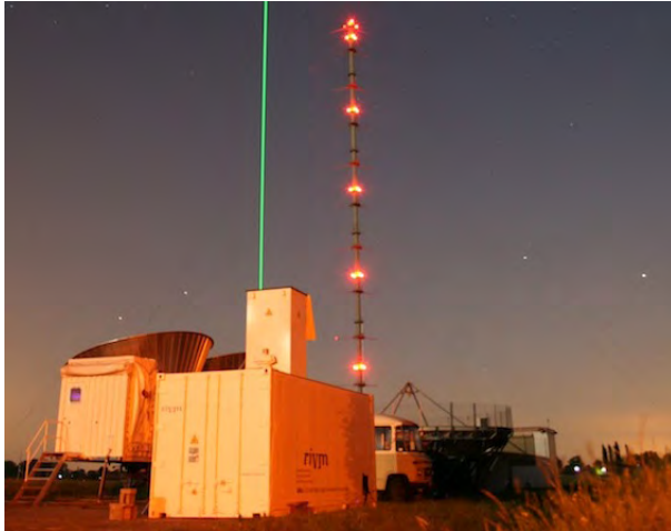
Figure 1: The Raman lidar Caeli in operation at the Cabauw Experimental Site for Atmospheric Research (CESAR), close to the 213 m high meteorological tower.
