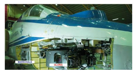
Figure 5.9. The GLORIA imaging FTS and the MARSCHALS millimetre-wave radiometer as accommodated inside the Geophysica aircraft.
