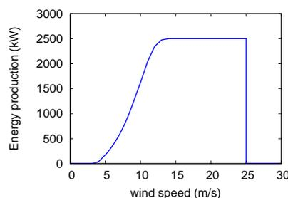
Figure 3. Power-curve wind turbine Nordex N-90
