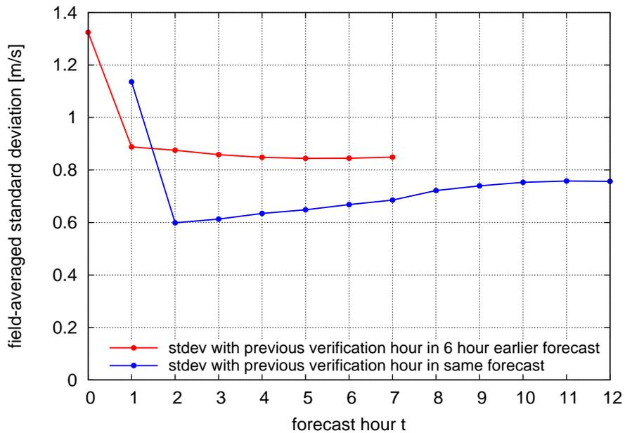
Figure 3.7: Field-averaged standard deviation of the point-wise difference of the wind speed in succeeding verification hours. Blue: based on fields within the same forecast runs; Red: based on fields which differ 6 hours in forecast time.
