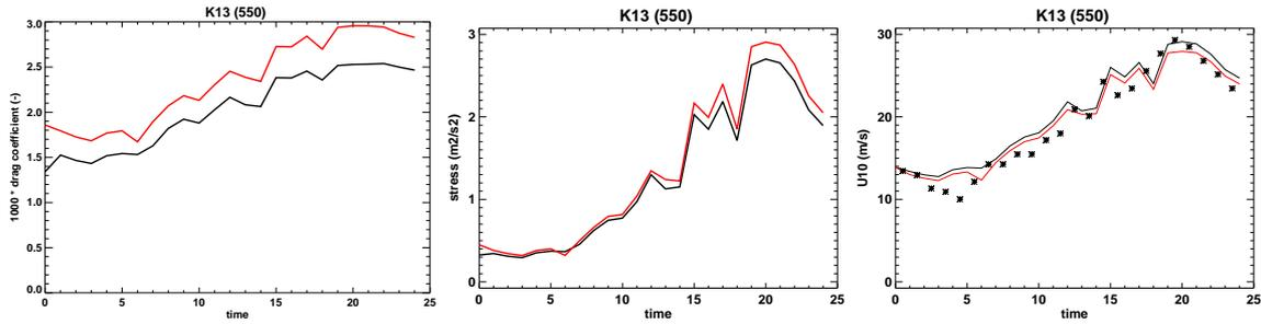
Figure 3.9: *HARMONIE* timeseries of the drag coefficient (left), surface stress (middle) and 10-m wind speed (right) for K13 for 25 Jan 1990. The black lines represent the reference simulation, the red lines represents a simulation with enhanced drag coefficients. For the wind speed, observations are added (symbols).
