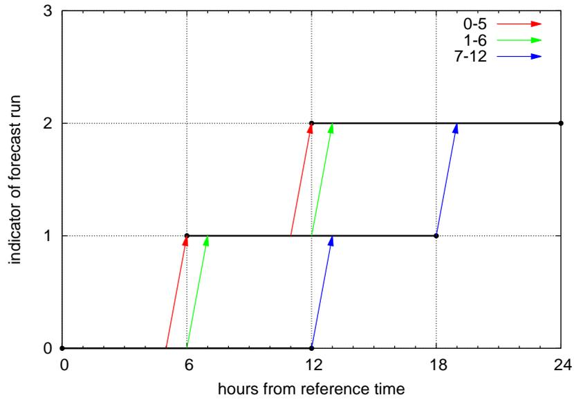
Figure 3.6: Schematic view of the concatenation of 6-hourly HARMONIE forecasts. The red arrows indicate that from every forecast run, the forecast hours 0 to 5 are used, implying no spin-up-time; the green arrows imply a spin-up time of 1 hour, using forecast hours 1 to 6, whereas a spin-up time of 7 hours are indicated by the blue arrows.
