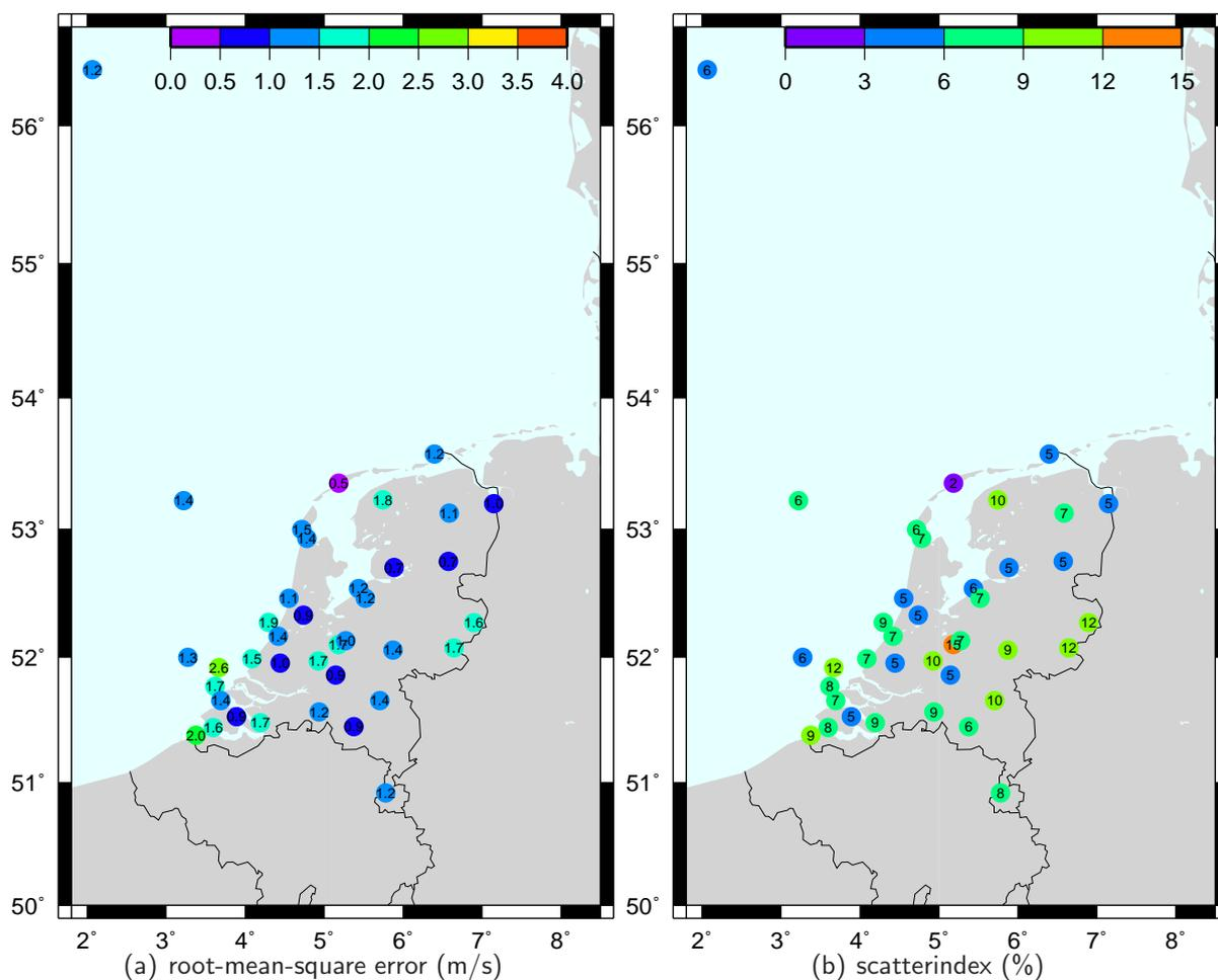
Figure 4.5: Left: Root-mean-square error in m/s (left) and scatterindex in % (right) of the modelled maximum wind speeds for the optimal gridpoint.
