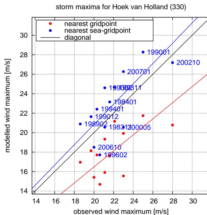
Figure 4.1: Scatterplot of the modelled and observed hourly wind maximum per storm for two gridpoints near Hoek van Holland. Red: nearest gridpoint; Blue: nearest sea-gridpoint. The year and month of the storms are plotted. The 197902 event is missing due to lacking observational data.
