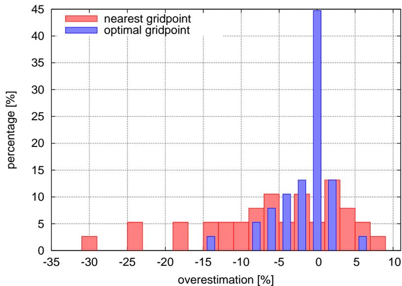
Figure 4.4: Histograms of the percentual overestimation of the maxima per storm for the nearest gridpoint (red) and the optimal gridpoint (blue). The optimal gridpoint is required to be less than 7.5 km (3 gridpoints) from the observational coordinates.
