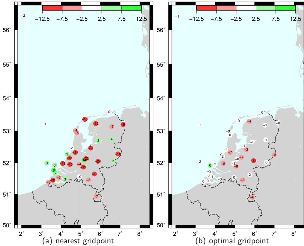
Figure 4.3: Percentual overestimation of the maximum wind speed per storm for the nearest gridpoint (left) and the optimal gridpoint for all measuring locations. The optimal gridpoint is required to be less than 7.5 km (3 gridpoints) from the observational coordinates.
