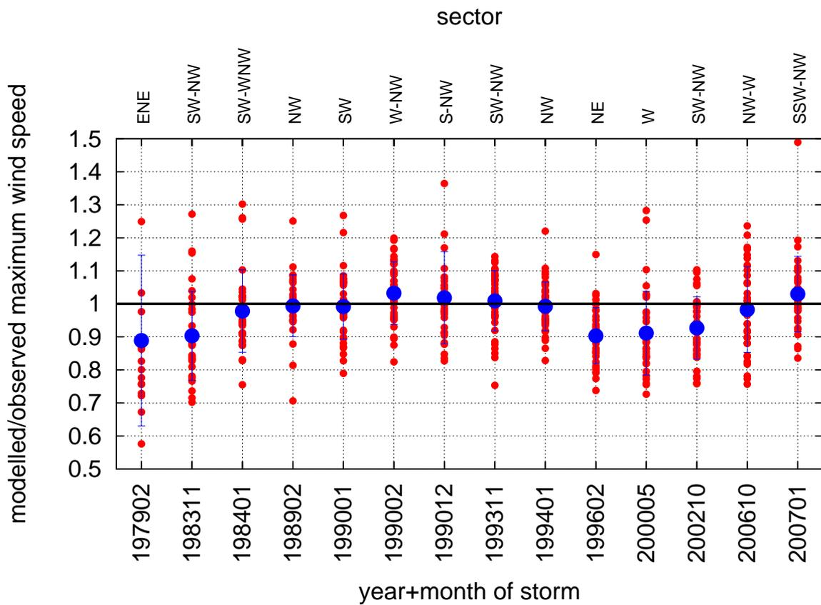
Figure 4.8: Ratio between modelled and observed wind speed per storm and per location (red). The average and standard deviation per storm are indicated in blue. The upper axis shows the dominant wind direction in The Netherlands. These wind directions are obtained from Table 3.1 of Groen and Caires (2011).
