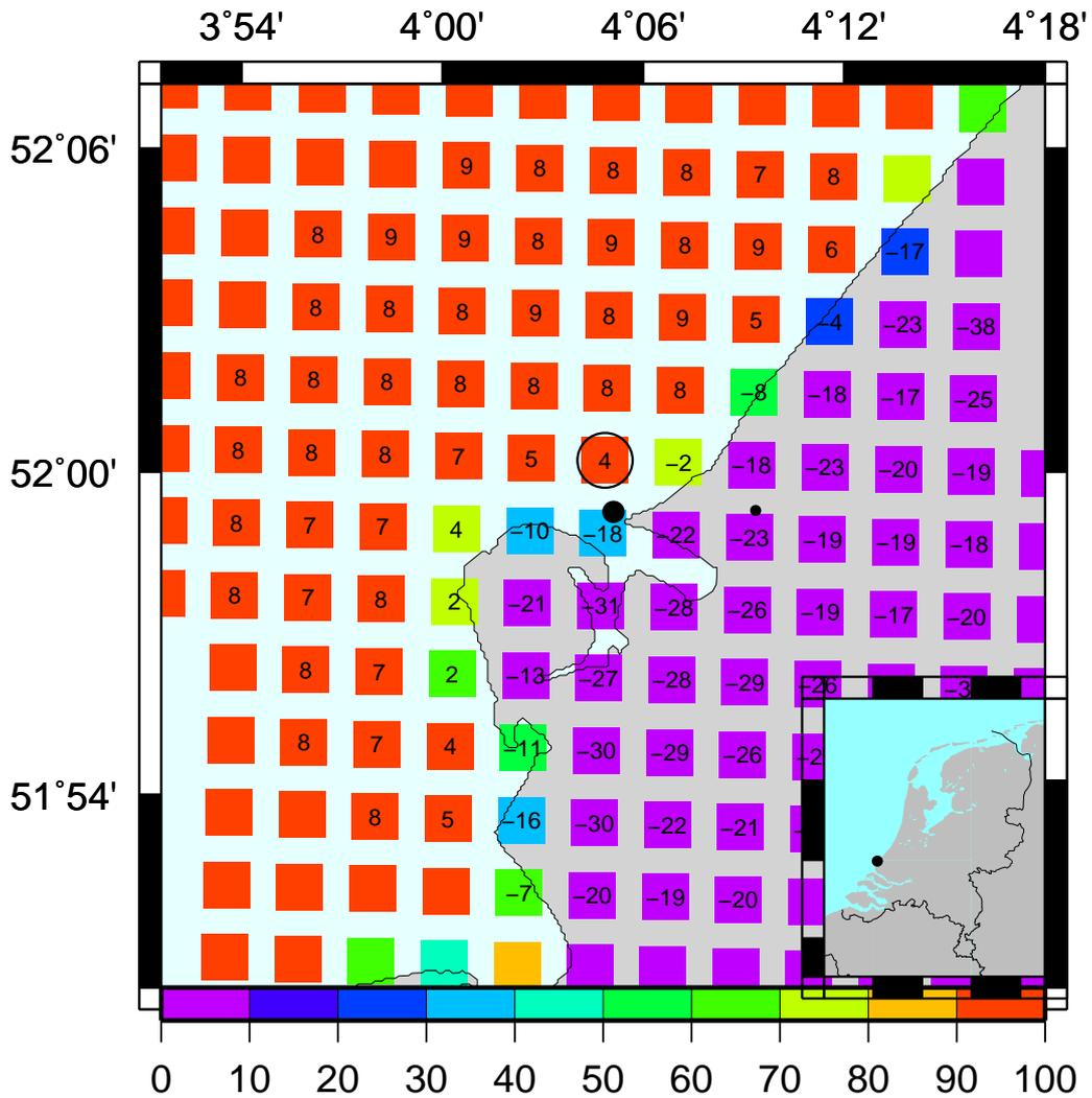
Figure 4.2: Percentual overestimation per gridpoint of the maxima per storm compared with the observations at Hoek van Holland. The colors indicate the percentage sea for every gridbox. The encircled number indicates the gridpoint with the nearest sea-gridpoint.
