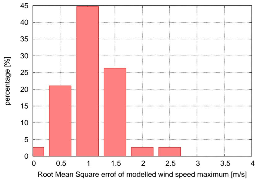
Figure 4.6: Histogram of the root-mean-square errors of the modelled maximum wind speed per storm for the optimal gridpoints.
