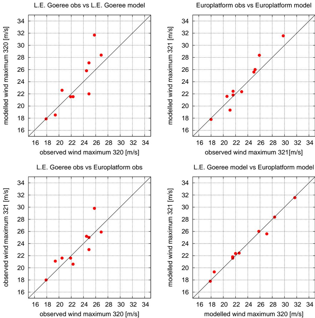
Figure 4.7: Scatterplots for Lichteiland Goeree (320) and Europlatform (321). The upper graphs show the modelled versus the observed maxima per storm for L.E. Goeree and Europlatform respectively; the lower graphs show the intercomparison of the stations for the observations and the model respectively.
