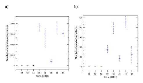
*Figure 2: a) Number of ASCAT data points read into the model and b) number of ASCAT data points used in the data assimilation on each cycle. The horisontal line marks the average number, and the vertical dashed bars the range for each model cycle.*
