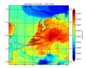
*Fig. 6.* Line along which the vertical slice of the RH is taken. Starting at the star above sea (left hand side of the vertical slice plot) and ending at the pentagon above land. Note that the flow is from the land (right) to the left (sea). Plotted is the specific humidity [kg/kg] at the lowest model level.
