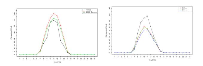
Figure 4. Simulated (left) and observed (right) time series of downward short wave radiation on the surface on 30<sup>th</sup> November 2011. Model values are horizontally averaged on a 1°x1° box, which includes the ground measurements plotted on the right panel. Note the scale difference of the vertical axes between the two plots.
