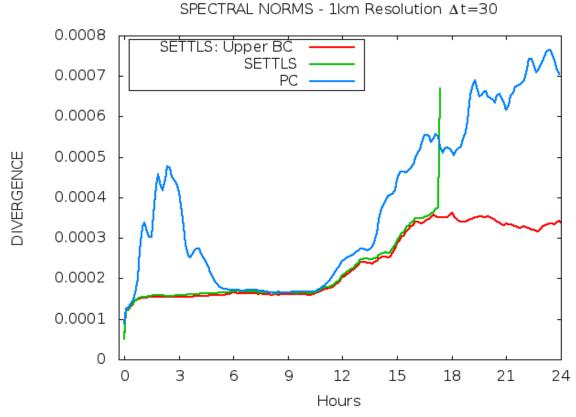
Fig. 4: Evolution of the vertically averaged horizontal divergence spectral norms for the three runs.
