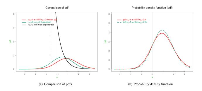
Figure 4: Plots of the probability density function. In 4(a) it is shown the exponential and the gaussian function as well as the convolution function of both of them. In 4(b) two pdf obtained by the convolution for different parameters.
