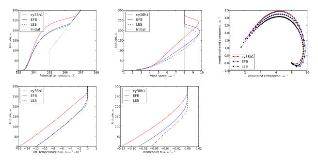
Figure 1: Profiles of potential temperature, wind speed, heat flux, momentum flux, and a hodograph, plotted nine hours after the initial time in GABLS1. MUSC cy38h1 is shown in red, MUSC with the EFBclosure in blue, and LES in black. The initial profiles of potential temperature and wind speed are drawn as dotted lines.
