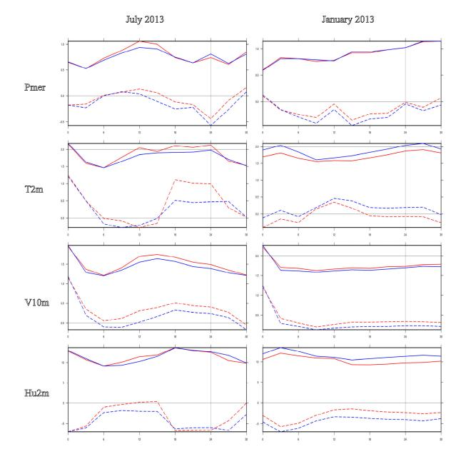
Figure 3: AROME surface scores of surface pressure(~150 obs), 2m temperature(~1000 obs), 10m wind speed (~700 obs) and 2m relative humidity (~800 obs) as a function of forecast step (in hours). AROME forecasts starts at 3TU, and are initialized and coupled with ARPEGE 0 TU forecasts. AROME-2,5km is in red, AROME-1,3km in blue. Left column July 2013, right column January 2013. Bias in dotted lines and RMSE in continuous lines.
