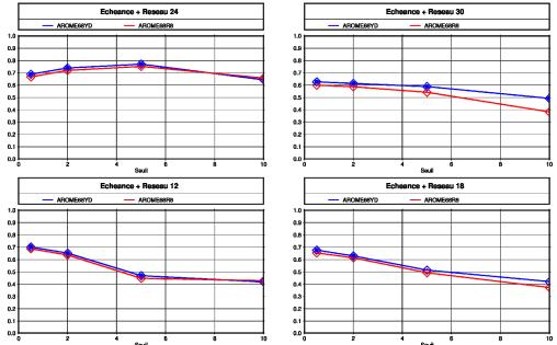
Figure 4a: Brier Skill Scores of 6h cumulated rainfalls with a neighbourhood of 20 km, as a function of precipitation thresholds (>0,2>2,>5 and >10 mm/6h), for 4 forecasts times (12 TU, 18 TU, 24 TU and 30=6 TU the next day).31 daily forecasts starting at 3 TU in January 2013 are used. AROME1,3km in blue, AROME 2,5km in red. Blue dots indicates statistically significant differences between the 2 curves.
