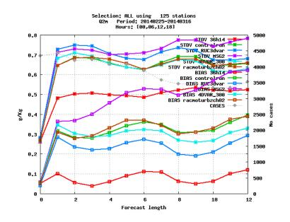
Fig. 10 Verification of  $q_{2m}$  [g/kg] of different Harmonie runs against EWGLAM stations. Shown are the bias and standard deviation as a function of the forecast period for the period from 20140225 to 20140316. Most important is the difference between the operational cycle 36h1.4 run (red) and the control run cycle 37h1.2 (green). Note that this period includes a cold start for the parallel runs.
