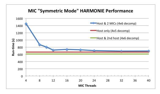
Figure 2: Total run-times 6-hr forecasts of the Ireland55 case, as in Fig. 1, when run in "symmetric" mode (diamonds), with 20 MPI tasks on the host node, and 2 on each of 2 MICs, as a function of MIC threads. Also shown is the host-only result (horizontal red line), and the result with 4 MPI tasks on a second host instead of on the 2 MICs (green line).
