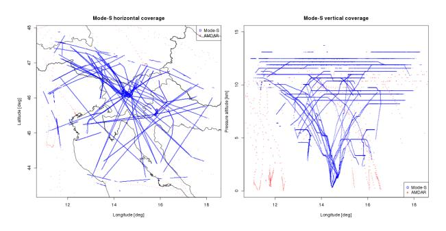
*Figure 1: An example of Mode-S MRAR horizontal and vertical coverage in 6 hours. The number of AMDAR observations is also shown.*
