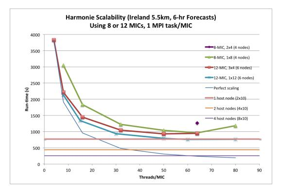
Figure 1: Run-times (s) for a 6-hr forecast of the HARMONIE IRELAND55 case, using 8 or 12 MICs, with 1 MPI task/MIC.
