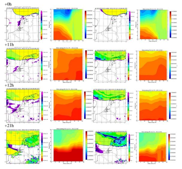
Fig. 7 Visibility plots [m] and vertical slices (lowest 8 model levels) of RH [0-1]along the line shown in Fig. 6. The left side of the vertical slice plots is located above sea and the right above land. The two columns on the left refer to standard runs and the two right columns refer to runs including the RACMO turbulence scheme and zch=0.2. The rows correspond with the forecast period as indicated.
