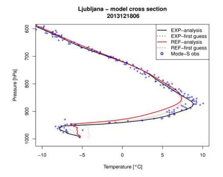
*Figure 2:* Impact of Mode-S MRAR on vertical temperature profile analysis. EXP is experiment with Mode-S observations, which are also shown as blue circles. Full lines are analysis profiles and dotted lines are first guess for the same analysis.
