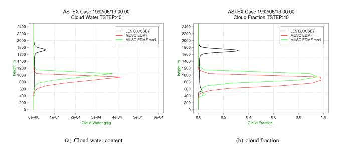
*Figure 1: Profiles of the cloud water content 1(a) and the cloud fraction 1(b) after 40 hours of simulation. Comparison of the MUSC reference (red lines), modified variance (green line) and LES (black line).*
