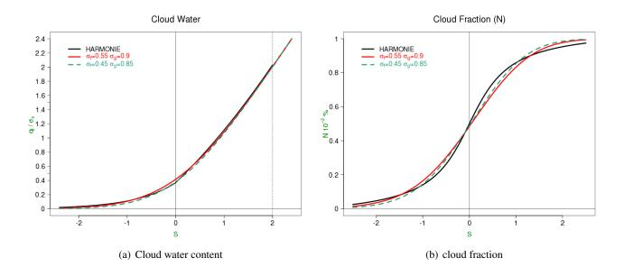
*Figure 5:* Plots of the cloud water content and the cloud fraction. In black the plot corresponding to the model, while in red and green the ones corresponding to the convolution pdf with  $\sigma_f = 0.55$ ,  $\sigma_g = 0.9$  (red) and  $\sigma_f = 0.45$ ,  $\sigma_g = 0.85$  (green)
