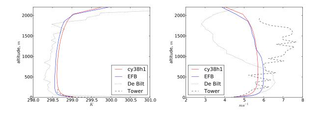
Figure 4: Potential temperature (left) and wind speed (right) at 12UTC on the 2nd of July 2006, 24 hours after the initial time in the GABLS3 experiments. MUSC cy38h1 is shown in red, MUSC with the EFBclosure in blue. Black dashed lines show data from the Cabauw tower (left) or wind profiler (right), dotted lines show the sounding at De Bilt some 30 km away.
