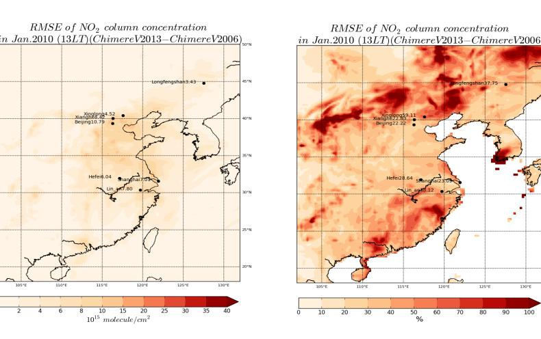
The RMSE of NO<sub>2</sub> column concentration between the old and new CHIMERE model helps us to check the model error estimates in DECSO. We can see that the high RMSE at the middle east part of China is related to high NO<sub>2</sub> concentrations. The high relative RMSE may be due to the added biogenic emissions in the new CHIMERE.
