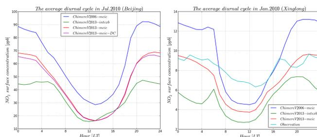
The diurnal cycle comparisons over Beijing and Xinglong show that the pattern of the different simulations is very similar. The deep convection option in the model has little effect. At Xinglong station, all the simulations underestimate the NO<sub>2</sub> surface concentration during day time as compared with the ground measurements. The NO<sub>2</sub> diurnal cycle of CHIMERE V2013 with MEIC is closest to the ground measurements.
