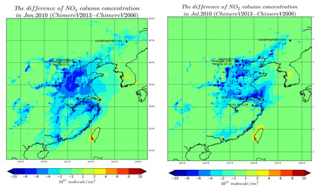
The NO<sub>2</sub> column concentration of CHIMERE V2013 is lower than that of CHIMERE V2006, especially over the highly polluted regions. This is because CHIMERE V2013 has a new transport scheme and secondary organic aerosol chemistry. In addition, its chemical reaction rates are updated.
