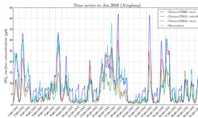
The time series figure above shows that both models have the capacity to simulate the diurnal cycle. Especially during night time, CHIMERE V2013 gives better results. CHIMERE V2006 overestimates the nocturnal NO<sub>2</sub> concentration at surface.
