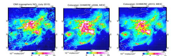
The comparison with the OMI satellite measurements shows that CHIMERE V2006 overestimate the NO<sub>2</sub> column concentration, while CHIMERE V2013 is closer to the observation.
