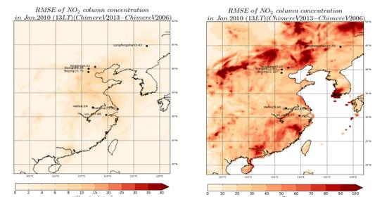
The RMSE of NO<sub>2</sub> column concentration between the old and new CHIMERE model helps us to check the model error estimates in DECSO. We can see that the high RMSE at the middle east part of China is related to high NO<sub>2</sub> concentrations. The high relative RMSE may be due to the added biogenic emissions in the new CHIMERE.
