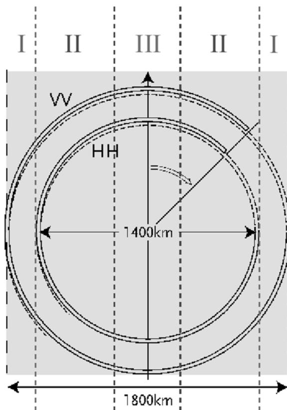
**Figure 1: Earth surface coverage of the scans of the horizontal (HH) and vertical polarisation (VV) pencil-beams of SeaWinds. As the satellite propagates towards the top of the page the swath (in grey) is illuminated, and three areas are discriminated:**
