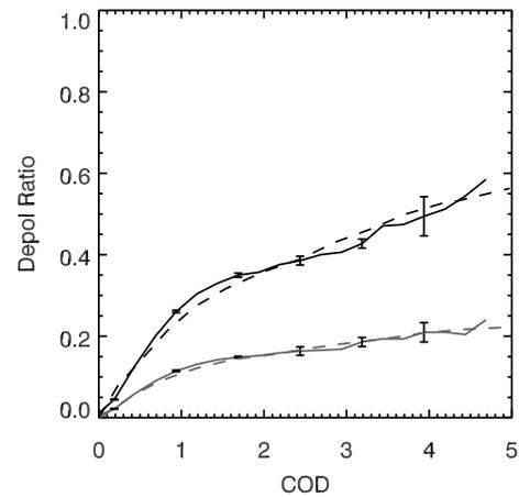
**Figure A2.** Linear and circular depolarisation profiles in a C1 cloud at a distance of 2 km for a FOV of 1.75 mrad and a wavelength of 700 nm as a function of cloud optical depth (COD). The solid line shows the ECSIM results while the dashed lines show the results calculated using an approximate analytical approach (Chaikovskaya, 2008).
