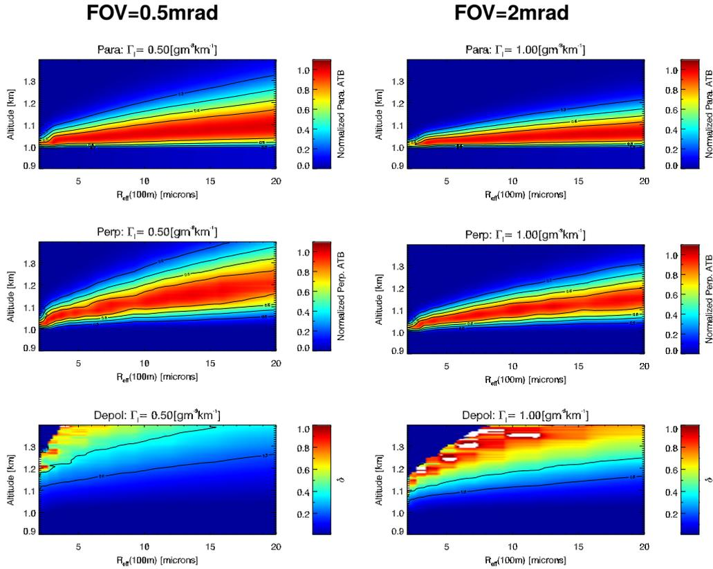
**Figure 3.** Example results of MC calculations for a lidar wavelength of 355 nm corresponding to semi-infinite clouds with a cloud-base of 1.0 km for two values of  $\Gamma_1$  as a function of  $R_{\text{eff},100}$  for lidar FOVs of 0.5 and 2.0 mrad. Here, for each value of  $R_{\text{eff},100}$ , the para and perp attenuated backscatter (ATB) values have been normalised by the maximum para return.
