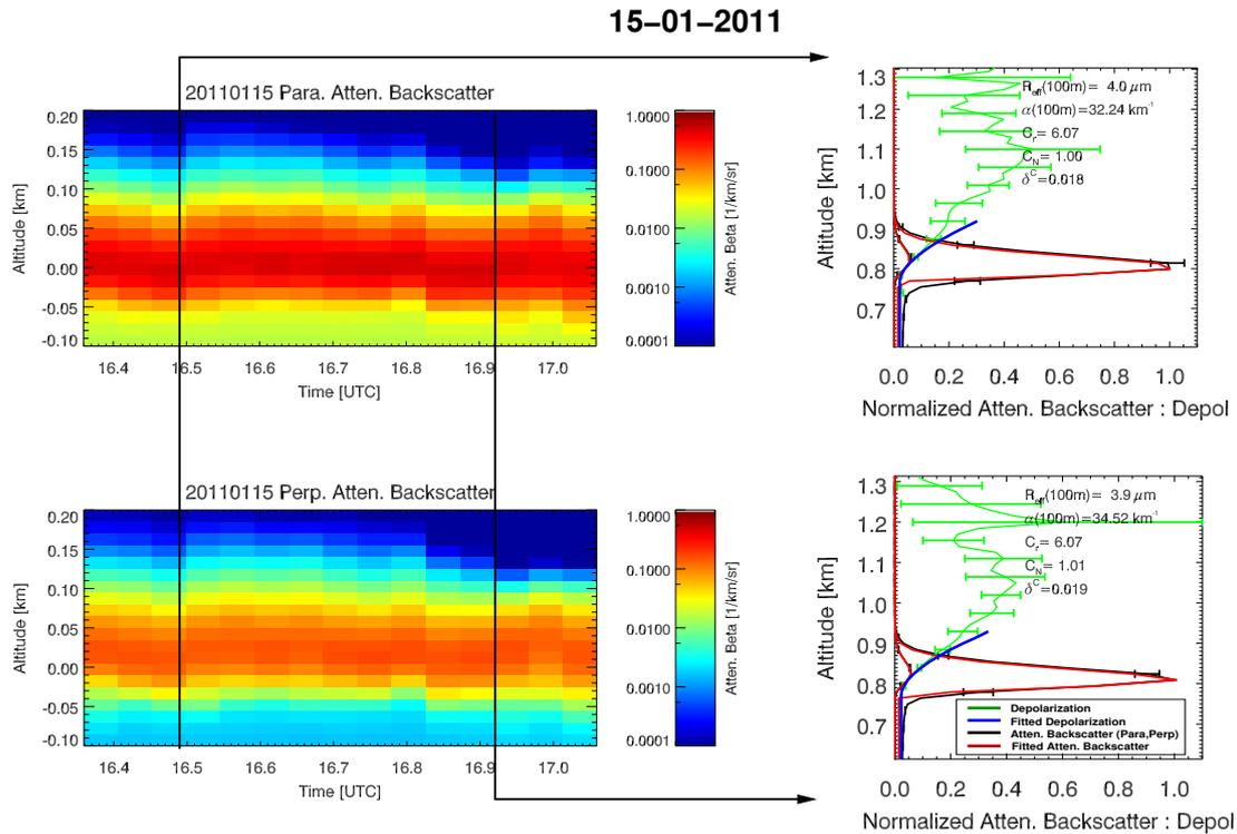
**Figure 14.** Normalised parallel and perpendicular attenuated backscatters as a function of altitude from the peak of the observed parallel backscatter profile (left panels) corresponding to the data shown in Fig. 13. Example fit results are shown on the right for 16.49 and 16.92 UTC.
