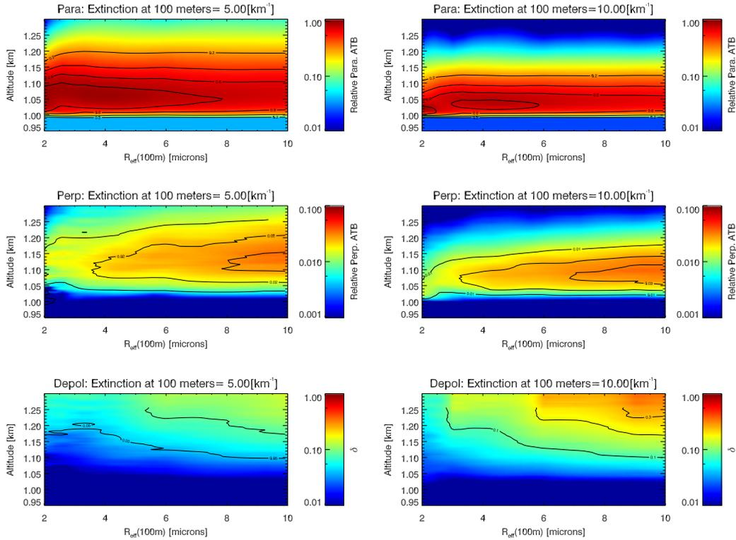
**Figure 4.** Example results of MC calculations for a lidar wavelength of 355 nm corresponding to semi-infinite clouds with a cloud-base of 1.0 km for two values of  $\alpha_{100}$  as a function of  $R_{\text{eff},100}$  for a lidar FOV of 1.0 mrad.
