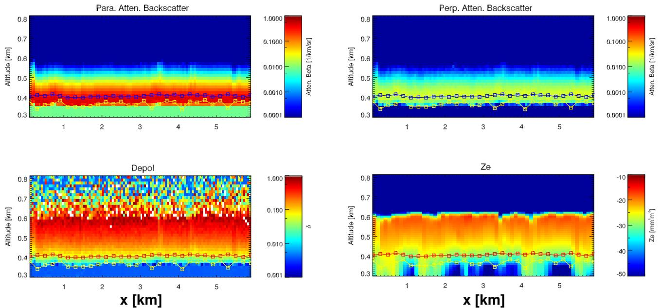
**Figure 9.** Simulated parallel and perpendicular attenuated backscatter signals for a 355 nm depolarisation lidar with a FOV of 1 mrad. Also shown are the corresponding linear depolarisation ratio and the radar reflectivity ( $Z_e$ ).
