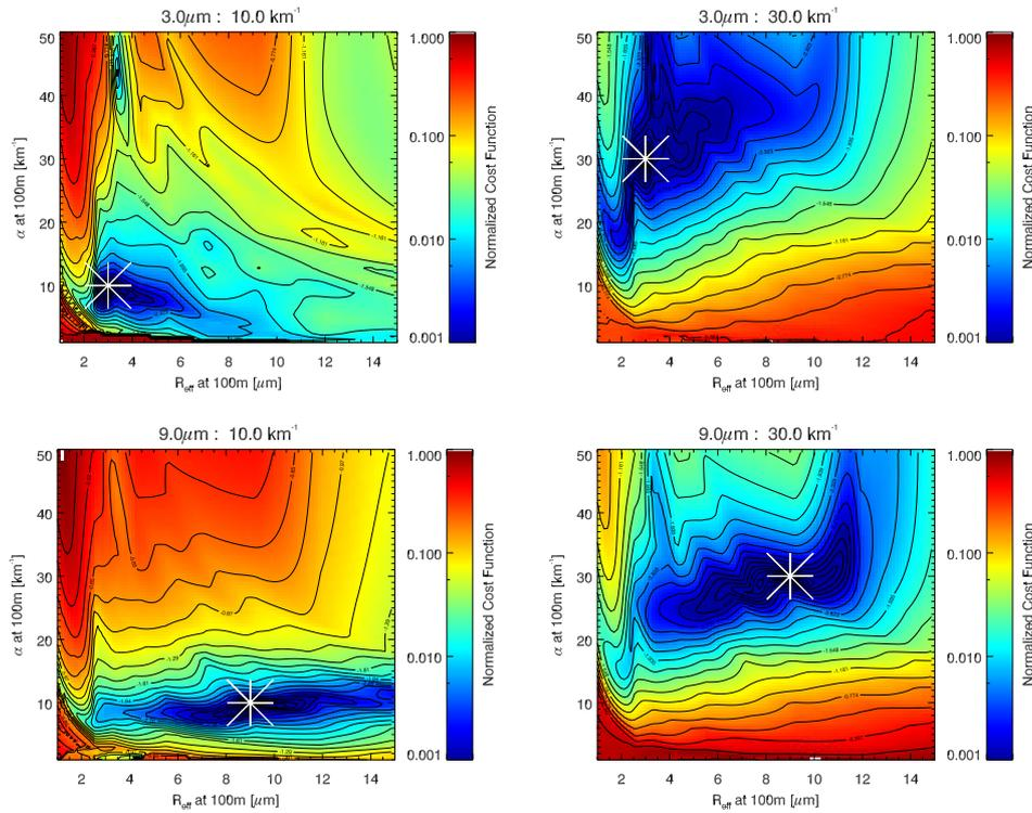
**Figure 5.** Normalised results from the application of Eq. (20) for a lidar wavelength of 355 nm as a function of  $\alpha_{100,k}$  and  $R_{\text{eff},100,k}$  for two true values of  $\alpha_{100}$  and  $R_{\text{eff},100}$  (as indicated) for a lidar FOV of 1.0 mrad and a cloud base of 1 km. The symbol is used to mark the location of the minimum of the cost function.
