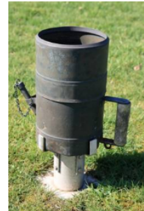
Figure 2.3: Example of a manual gauge (with the rim at 0.4 m).
