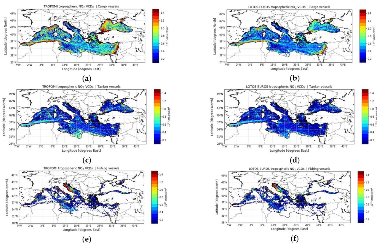
**Figure 8.** Tropospheric NO<sub>2</sub> vertical column densities (in  $10^{15}$  molecules  $\text{cm}^{-2}$ ) classified according to the 2019 vessel density per vessel type: (a) TROPOMI cargo; (b) LOTOS-EUROS cargo; (c) TROPOMI tanker; (d) LOTOS-EUROS tanker; (e) TROPOMI fishing; (f) LOTOS-EUROS fishing.
