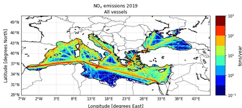
**Figure 3.** CAMS-GLOB-SHIP v2.1 2019 NO<sub>x</sub> emissions (tons per year).
