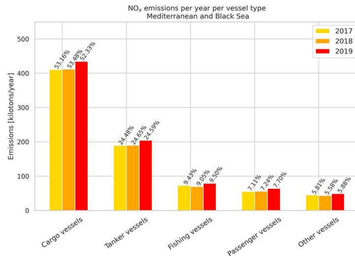
**Figure 6.** CAMS-GLOB-SHIP NO<sub>x</sub> emissions (in kilotons y<sup>-1</sup>) per vessel type and year in the Mediterranean and the Black Sea.
