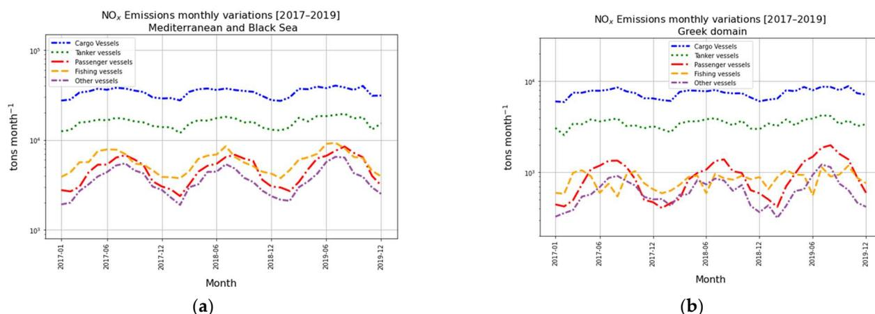
**Figure 7.** CAMS-GLOB-SHIP  $\text{NO}_x$  emissions time series from 2017 to 2019 (in tons per month) classified according to the EMODnet vessel density data of all the available years: Cargo vessels in blue, tanker vessels in green, fishing vessels in orange, passenger vessels in red and other vessels in purple; (a) Mediterranean and Black Sea; (b) Greek domain.
