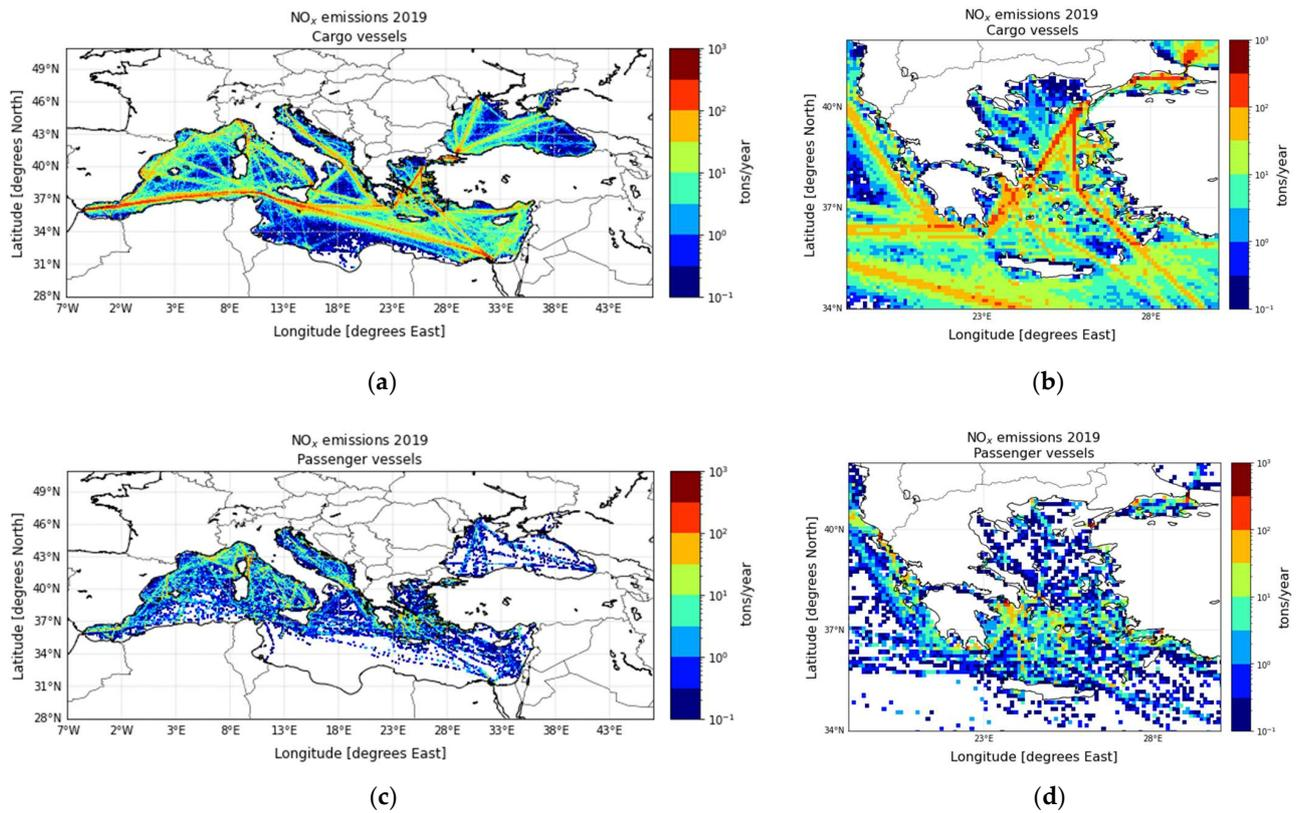
**Figure 5.** CAMS-GLOB-SHIP NO<sub>x</sub> emissions (in tons per year) classified according to the vessel density per vessel type: (a) Cargo vessels in the Mediterranean and the Black Sea; (b) Cargo vessels in the Greek domain; (c) Passenger vessels in the Mediterranean and the Black Sea; (d) Passenger vessels in the Greek domain.
