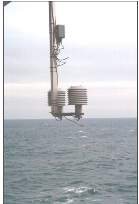
figure 2b: setup showing a dish screen at a sea station (Noordwijk measuring station)
