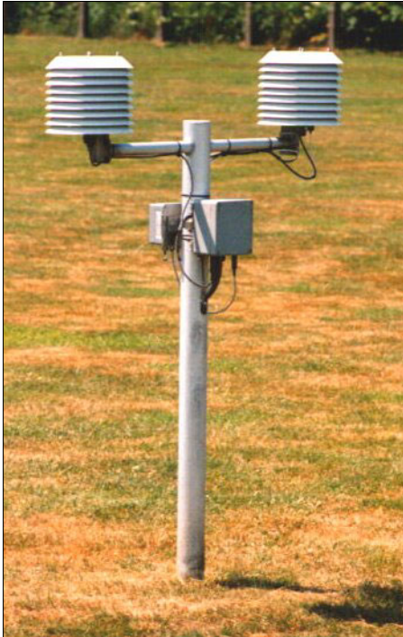
figure 2a: setup showing a dish screen at an inland station (De Bilt)
