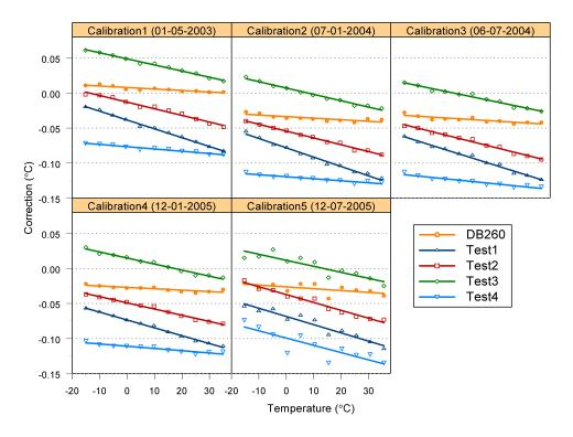
Figure A.1: Calibration curves of the PT-500 temperature sensors for the operational site DB260 and the 4 parallel sites, giving for each sensor the temperature correction as a function of temperature. Each panel represents a calibration: one at the beginning and end of the experiment and at three intermediate times. The symbols give the values as determined in the KNMI calibration lab, the lines present linear least-squares fits.
