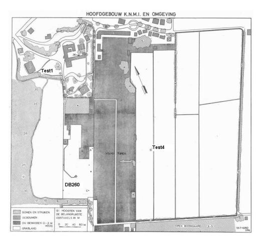
Figure 1.2: Plan of the KNMI observatory in 1960 indicating the tree height around the observation field. For comparison purposes the locations DB260, Test1 and Test4 are depicted on the map.
