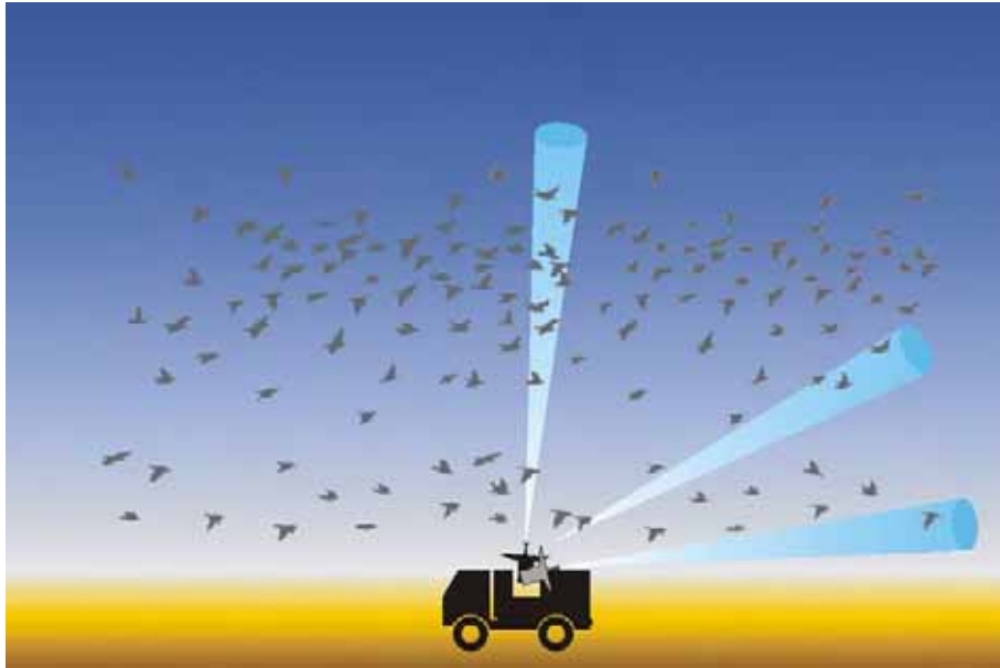
Figure 4.2: In the fix beam mode all objects showing up in the static beam are recorded. To get samples from relevant flight altitudes the measurement is repeated at different elevations (three in the case shown).
