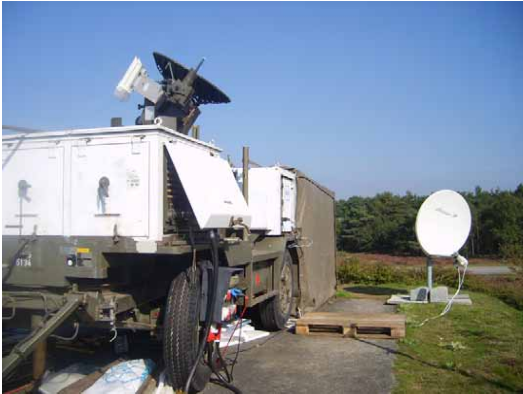
Figure 4.1: The Bird radar “Superfledermaus” equipped with a telescope and a camera mounted parallel to the radar antenna and a satellite connection for data transfer.
