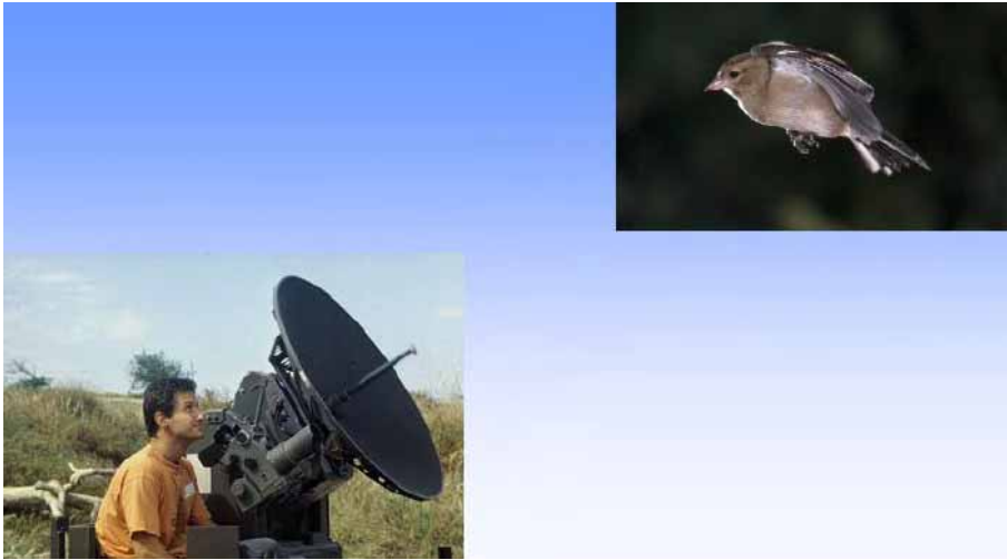
Figure 4.3: In the tracking mode the three dimensional flight path and the echo signature of a single target is recorded. During daytime an observer seeks to identify the target through a telescope mounted parallel to the radar antenna. During the night and with bad visibility (fog) only the echo signature is used to classify the targets.
