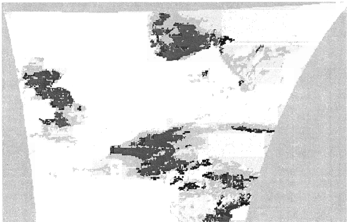
Figure 4: Example of a comparison of the current cloud detection algorithm with the MetCLOCK algorithm of Feijt et al (2000). Pixels are coloured according to the consistency with MetCLOCK: Light grey: both cloudy; light middle grey: MetCLOCK cloud free, present algorithm cloudy; dark middle grey: both cloud free; dark grey: MetCLOCK cloudy, present algorithm cloud free.
